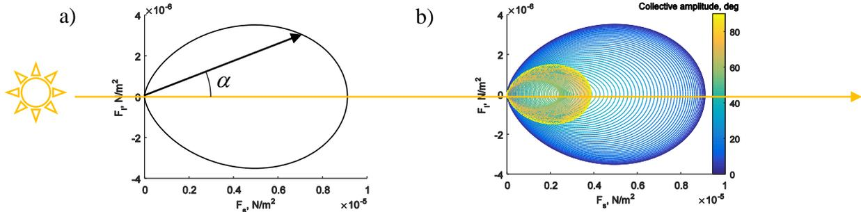
Figure 1 Solar sail “force bubble”. a) Flat solar sail. b) Heliogyro with collective profile.
