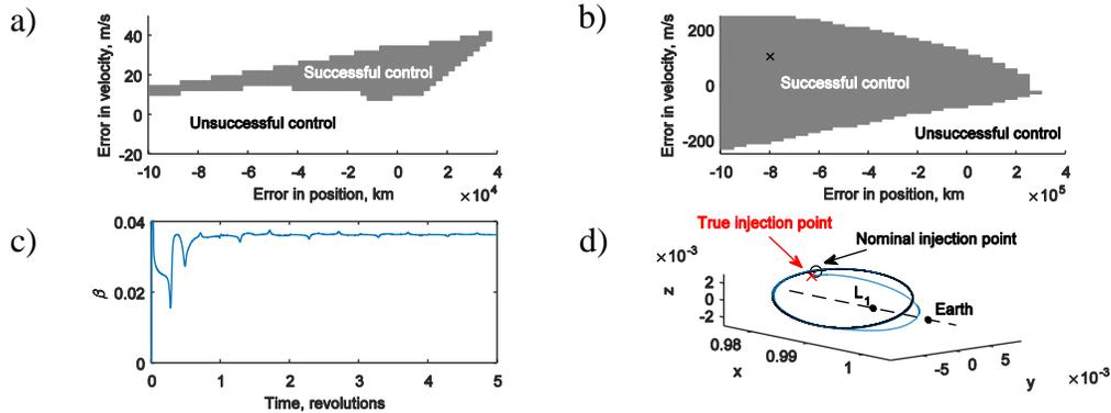
Figure 2 Solar sail halo orbit orbital control. a-b) Recoverable injection error for a flat sail (a) and heliogyro (b). c-d) Detailed results for black marker in plot b).
