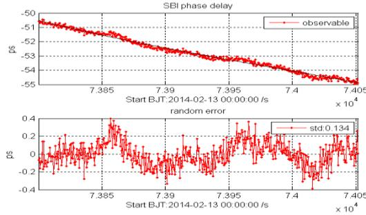
**Figure2. (a)SBI observing identify the movement of rover; (b)random error of SBI is 0.134 ps**
