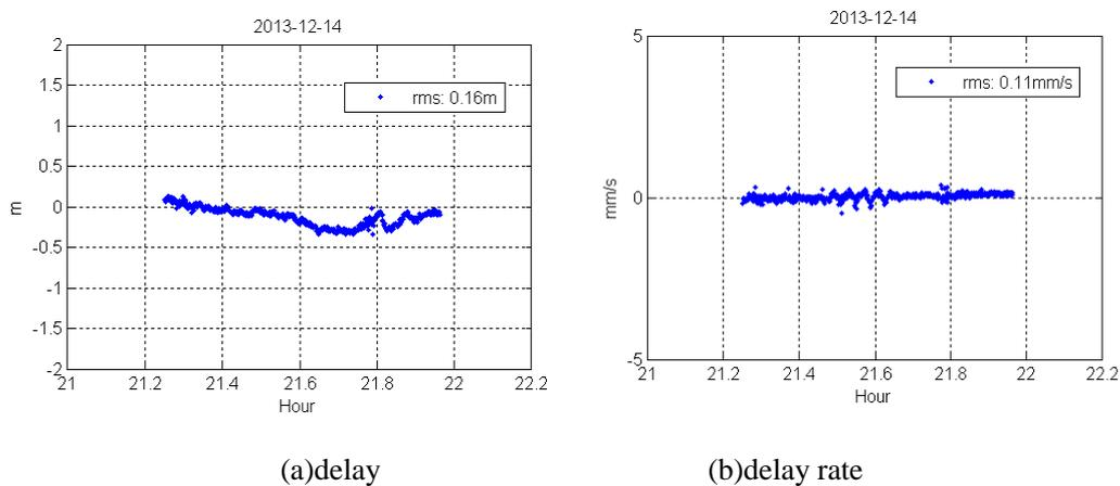
Figure 1. Delta-DOR tracking Observable Accuracy, the random error is about 0.5ns and 0.33ps/s corresponding  $(\Delta\tau, \Delta\dot{\tau})$
