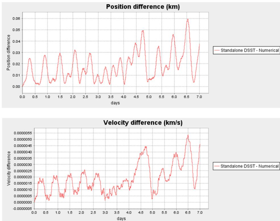
Figure 3 MEO (Galileo-like orbit)
