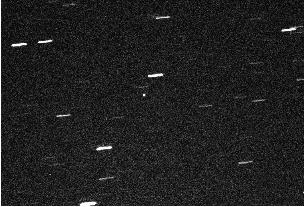
Figure 4. Typical picture of an observation night. An object can be identified as a spot (e. g. in the middle of the picture), stripes are identified as stars.
