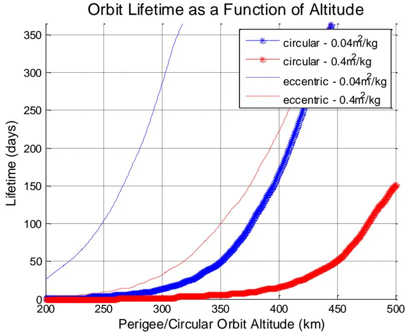
**Figure 1. Orbit Lifetime as a Function of Altitude**
