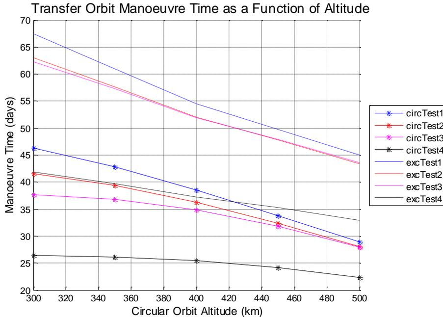
**Figure 3. Transfer Orbit Manoeuvre Time as a Function of Altitude**
