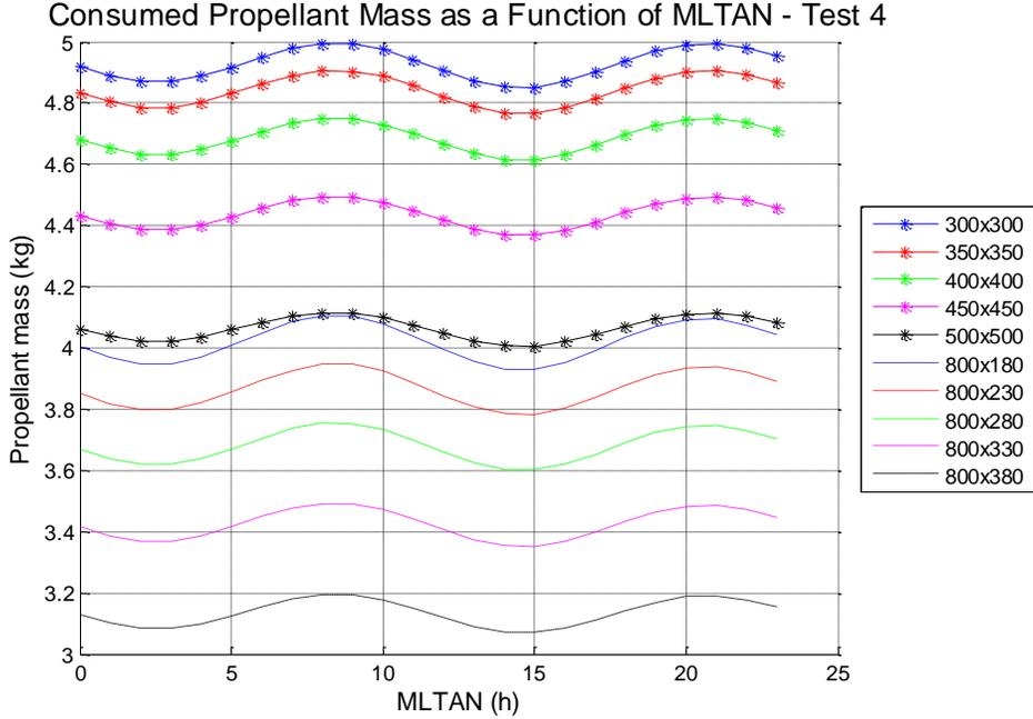
**Figure 5. Consumed Propellant Mass as a Function of MLTAN During Transfer - Test 4**
