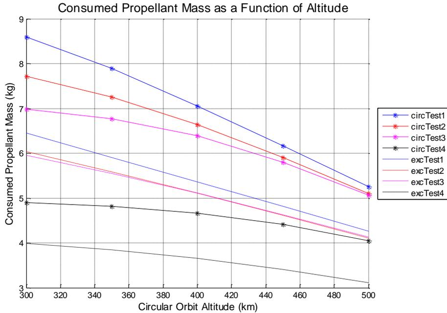
**Figure 4. Consumed Propellant Mass as a Function of Altitude**
