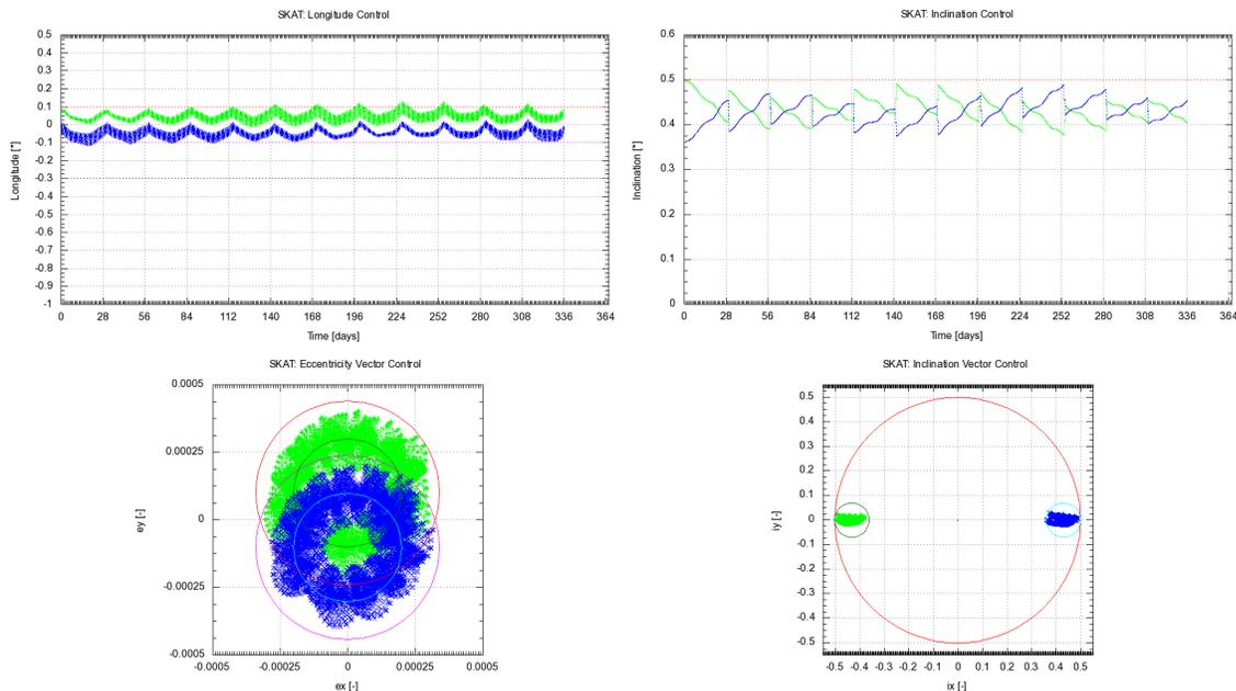
**Figure 3: Case 1f, 28 days cycle,  $\pm 4\%$  radial X-coupling, ecc.control, 12 hours between NS**
