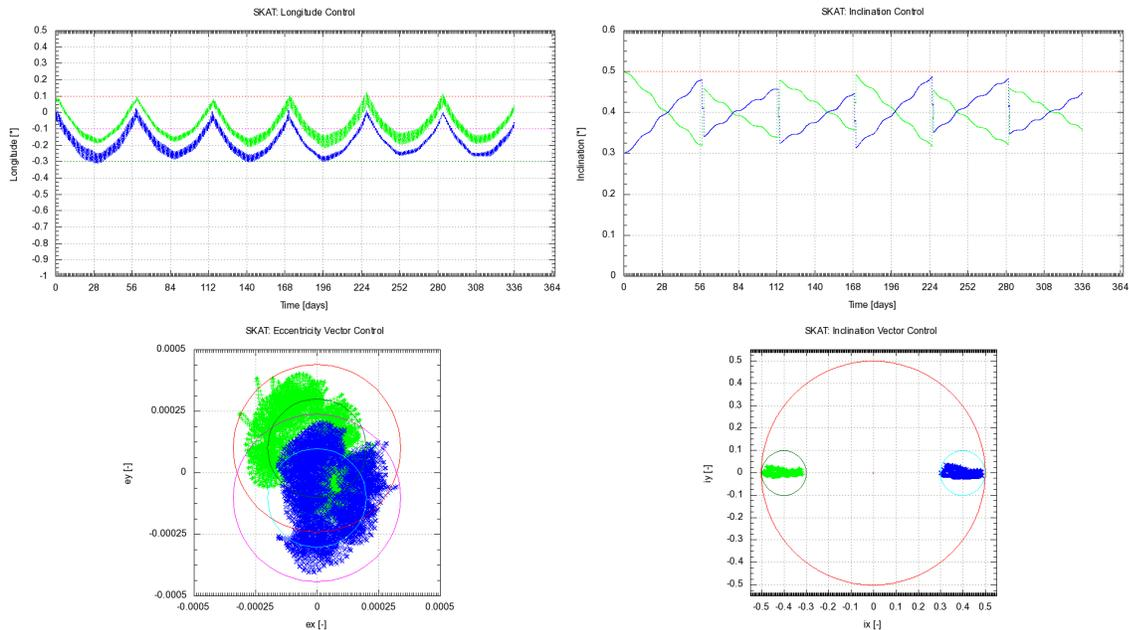
**Figure 4: Case 2d, 56 days cycle,  $\pm 4\%$  radial X-coupling, ecc.control, 24 hours between NS**
