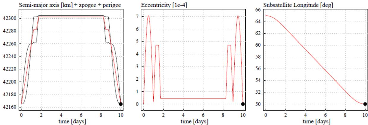
**Figure 9. Time evolution of Keplerian elements for GEO relocation.**
