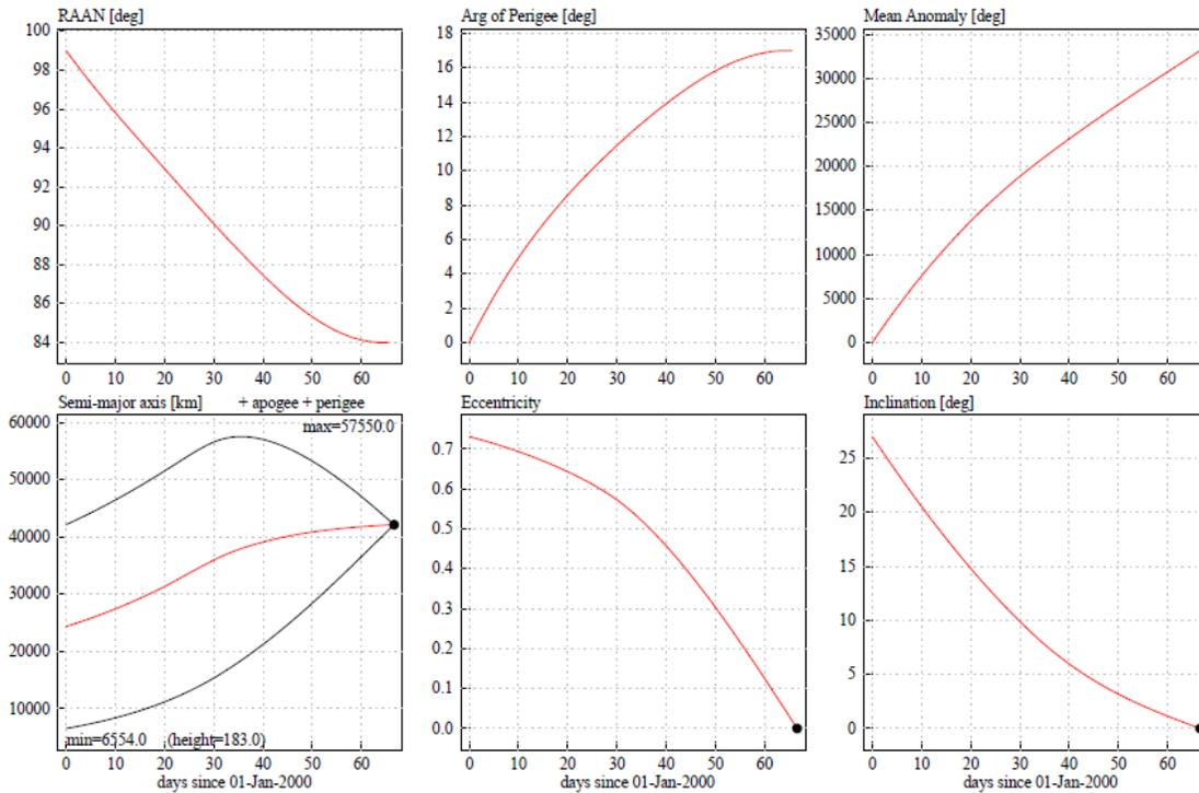
**Figure 2. Keplerian elements for Case 4 (GTO to GEO)**
