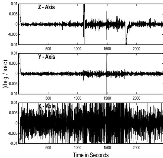
**Fig. 2:** The Error Between the Raw Angular Rate,  $\underline{\omega}_r$ , and the Nominal Angular-Rate.
