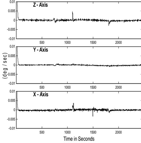
**Fig. 5:** The Estimated Angular-Rate,  $\hat{\omega}$ , After Applying the PSELIKA Filter to the Augmented Model.
