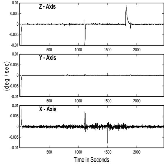
**Fig. 3:** The Error in the Estimated Angular-Rate,  $\hat{\underline{\omega}}$ , After the PSELIKA Filter was Applied to  $\underline{\omega}_r$ .
