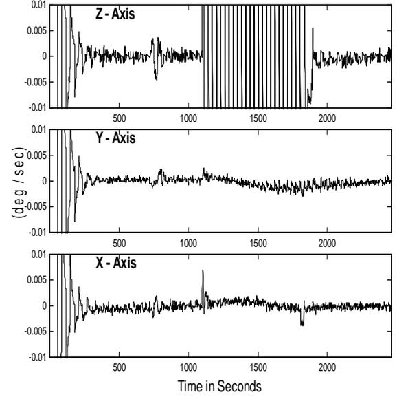
**Fig. 7:** The Estimated Angular-Rate Error After Applying the PSELIKA Filter to the Simplified Model with Sparse Measurements.
