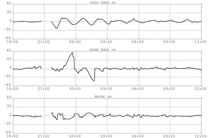
**Figure 3: DIODE-SPOT4 errors after a maneuver**
