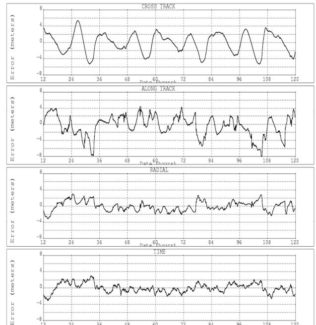
Figure 6: DIODE-GPS routine errors
