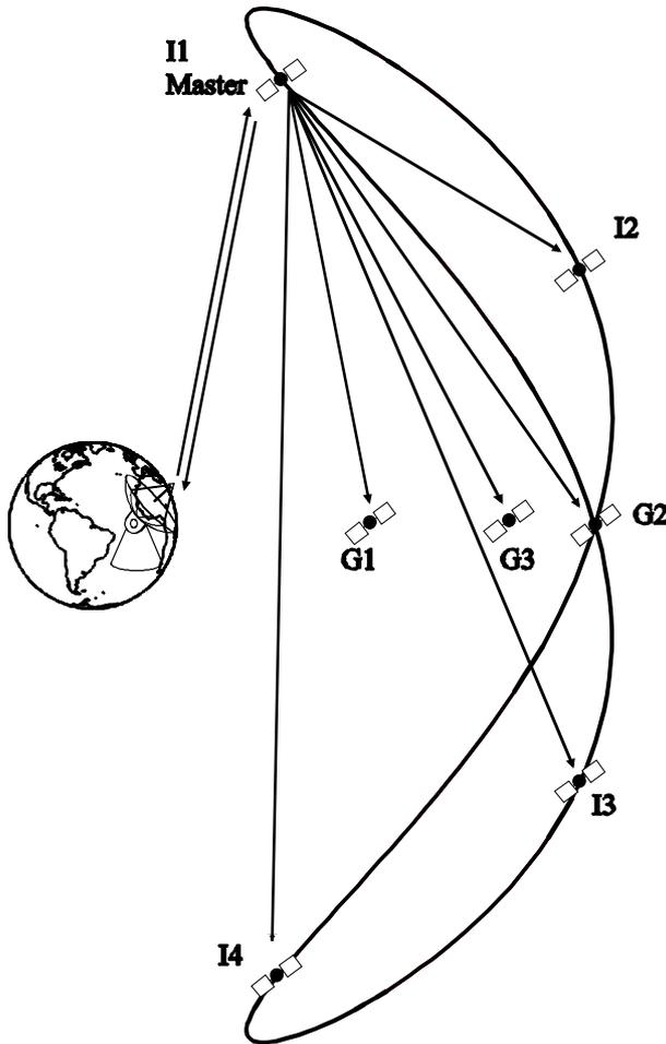
**Figure 4** GNSS-2 tracking with Master/Slave concept.
