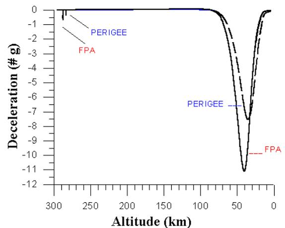
**Fig. 4 - Deceleration versus Altitude**
