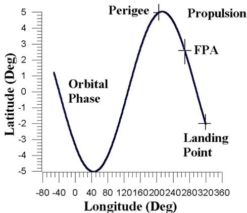
Figure 5 - Orbital phase, start time of reentry injection and Landing Point.
