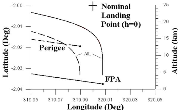
Figure 6 - Details of the trajectories of vehicle below 25 km for criteria FPA and *Perigee*.
