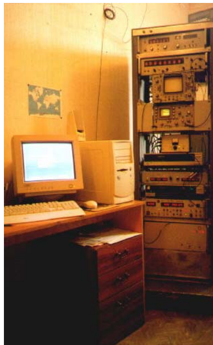
Fig. 3. NIRFI-3 correlator of Mk-2 format in Radio Physical Research Institute, N. Novgorod, Russia
