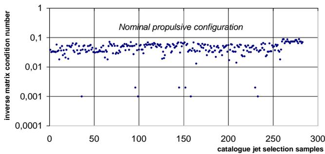
Figure 7 Inverse matrix condition number for each 6 jet selection
