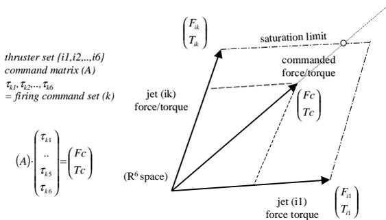
Figure 5 principle of linear saturation
