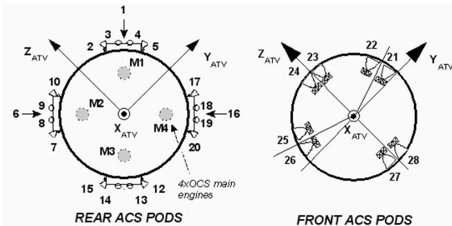
Figure 2 ATV Attitude Control System thrusters pods location
