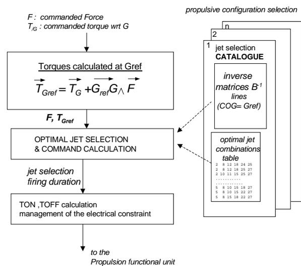
Figure 4 Functional synoptic of the optimal jet command by catalogue
