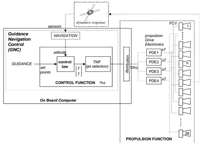
Figure 3 Vehicle control functional architecture
