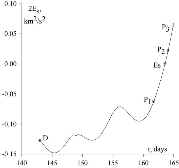
Fig. 3. Selenocentric energy versus the time for initial part of the Moon-to-Earth detour flight with escape from the lunar attraction
