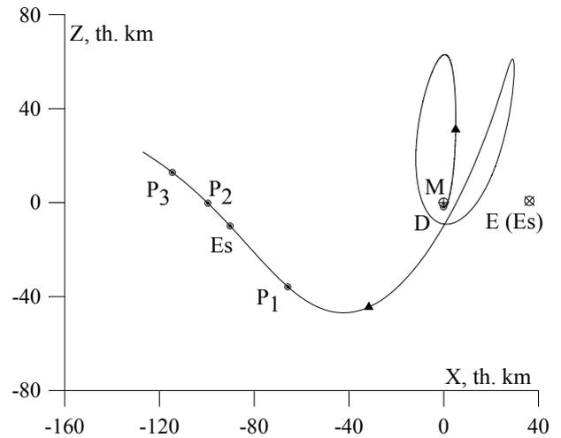
Fig. 2. The XZ view for the Moon-to-Earth selenocentric trajectory of detour type at initial part of the flight
