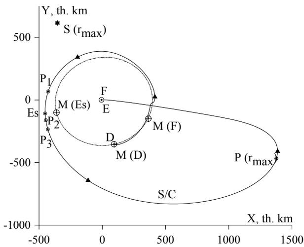
Fig. 1. The XY view for the Moon-to-Earth geocentric trajectory of detour flight
