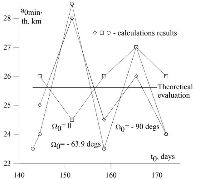
Fig.4. Minimal value of initial semimajor axis depending on the time of start from near-Moon elliptic selenocentric orbit for the Moon-to-Earth detour trajectories
