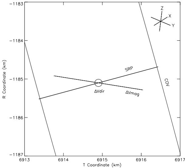
Figure 1: Three-sigma error ellipses for individual uncertainties: SRP (solar radiation pressure),  $\Delta V_{mag}$  (release  $\Delta V$  magnitude),  $\Delta V_{dir}$  (release  $\Delta V$  direction) and COV (initial state vector covariance information).
