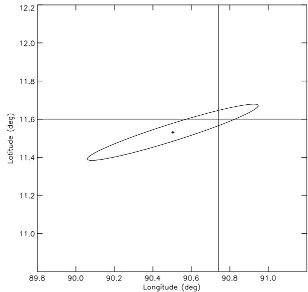
Figure 3: Reconstructed landing site and mapped three-sigma uncertainties onto the planetary surface. The nominal landing longitude and latitude are displayed.
