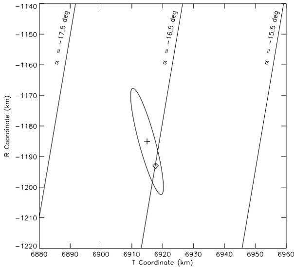
Figure 2: Reconstructed and nominal B-plane impact point with three-sigma error ellipse and allowed entry angle corridor.
