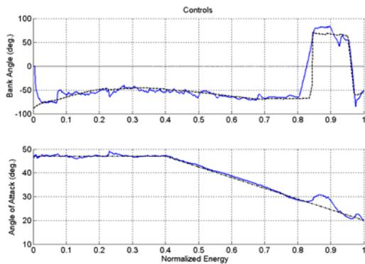
Fig. 2. Planned (dashed) and simulated (solid) bank and attack angle profiles
