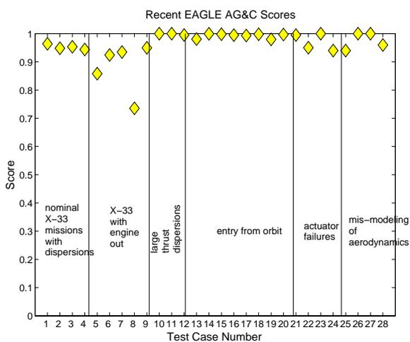
Fig. 6. Test results for dispersion and failure cases
