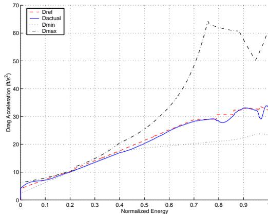
Fig. 1. Planned reference and simulated (actual) drag profiles within maximum and minimum drag boundaries
