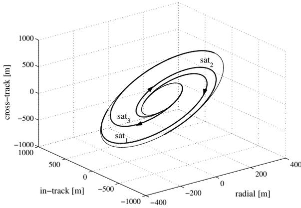
Fig. 3. Three satellites reconfiguration maneuver, circular reference orbit
