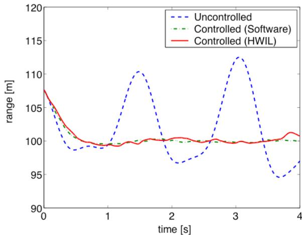
Fig. 2: Controlled and uncontrolled inter-spacecraft range, with proportional derivative control targeting 100m separation
