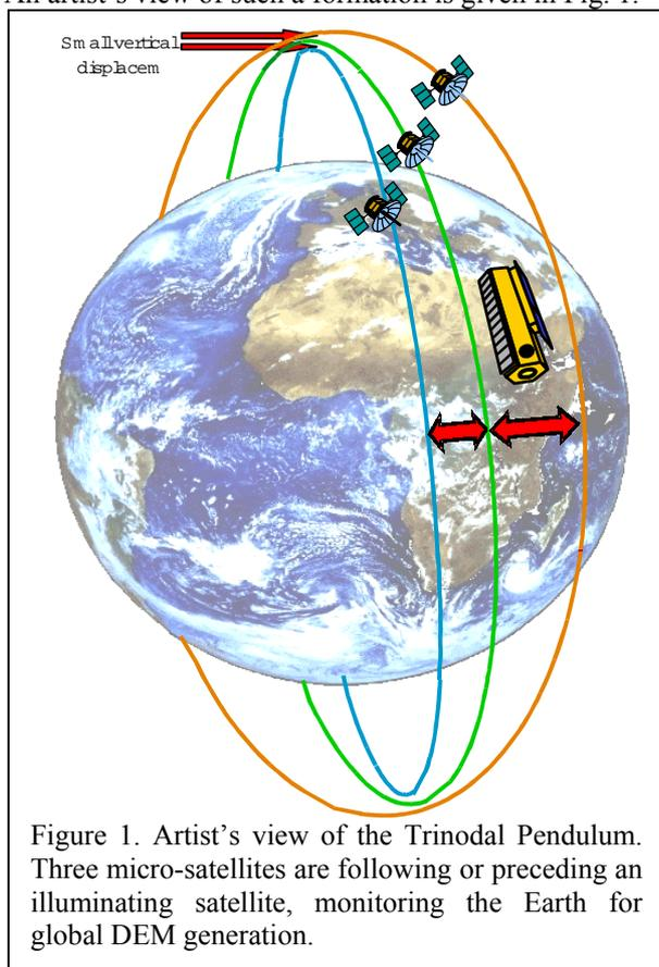
Figure 1. Artist's view of the Trinodal Pendulum. Three micro-satellites are following or preceding an illuminating satellite, monitoring the Earth for global DEM generation.
