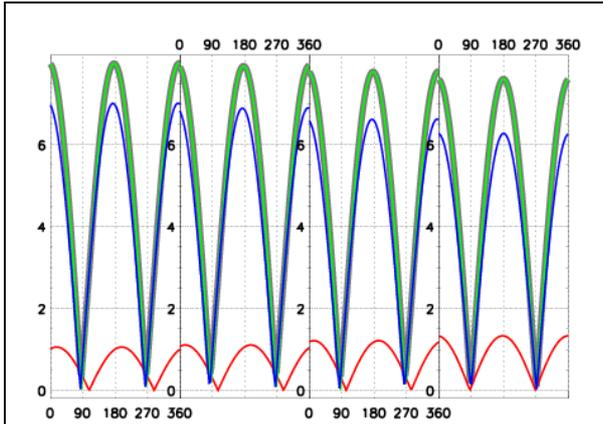
Figure 3. Effective baselines in [km] vs. argument of latitude. The effective baselines are very stable. We show the long time evolution of a whole orbit in the beginning, after 3 days, after 10 days and after 30 days. The different colors mark the different baselines between the micro-satellites. The stability is almost independent of solar flux activity. The small variations of the effective baselines are due to the difference in the respective eccentricity vectors.
