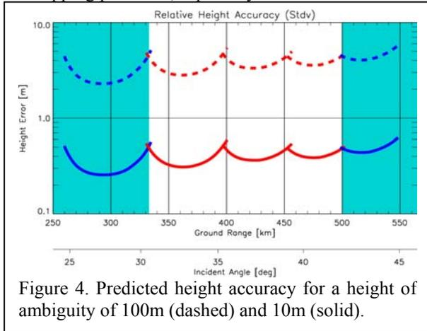
Figure 4. Predicted height accuracy for a height of ambiguity of 100m (dashed) and 10m (solid).
