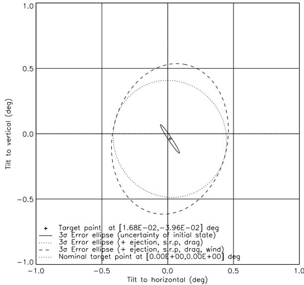
Fig. 1. Tilt of lander attitude w.r.t. relative velocity
