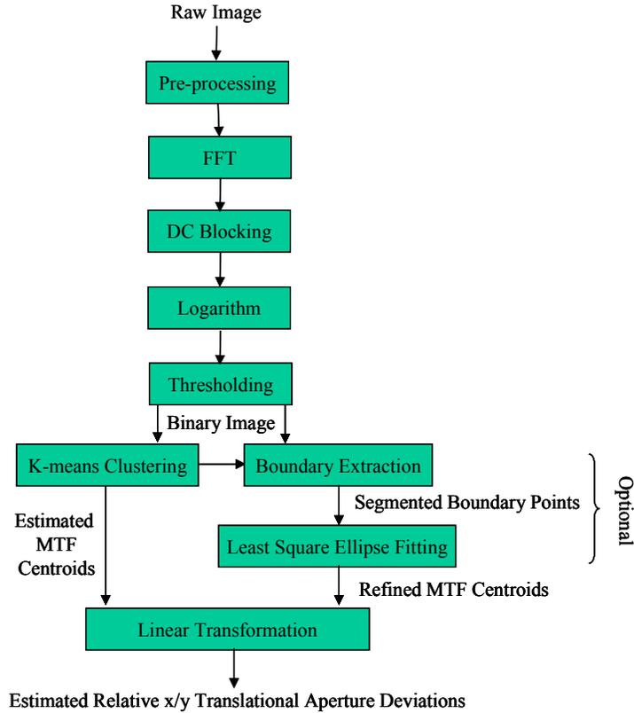
**Figure 7. Estimation Procedure of the x/y Translational Deviations**
