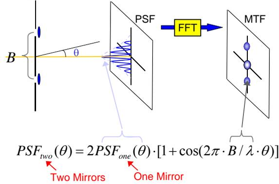
**Figure 4. PSF and MTF of a 2-Element Interferometer**
