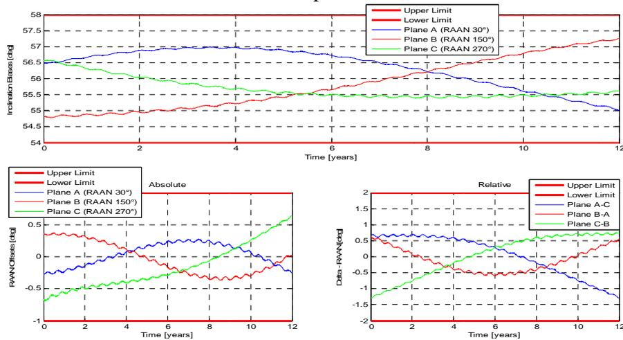
Fig. 7. Out-of-plane absolute optimization. Inclination (above). Absolute RAAN optimization (below left). RAAN differences between planes (below right).
