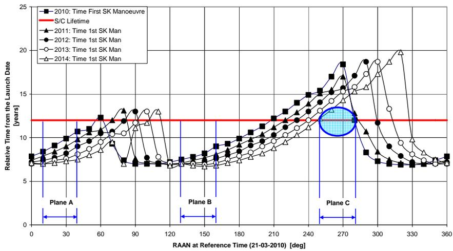
Fig 8. Time after launch for the first SK manoeuvre. Note that the abscise is RAAN value at  $T_o$ .
