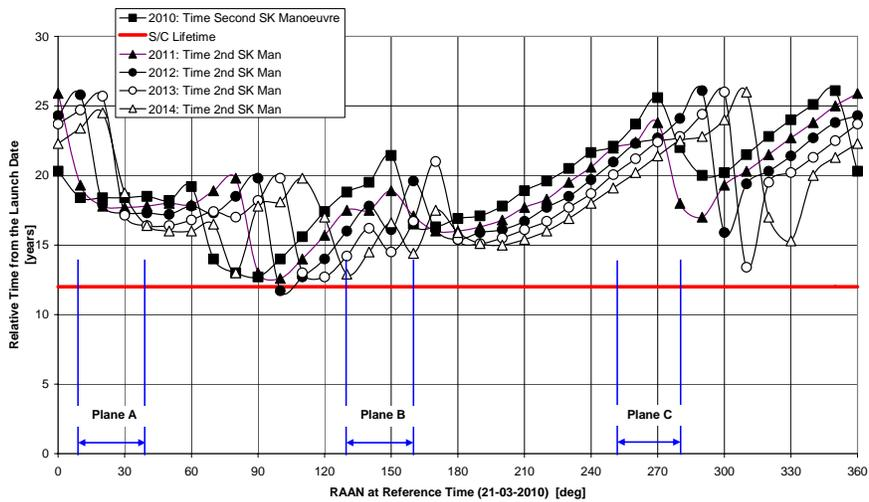
Fig 9. Time after launch for the first SK manoeuvre. Note that the abscise is RAAN value at  $T_o$ .
