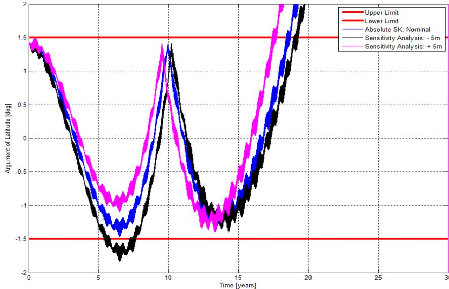
Fig. 10. Absolute in-plane optimization: Sensitivity to errors in semi-major axis
