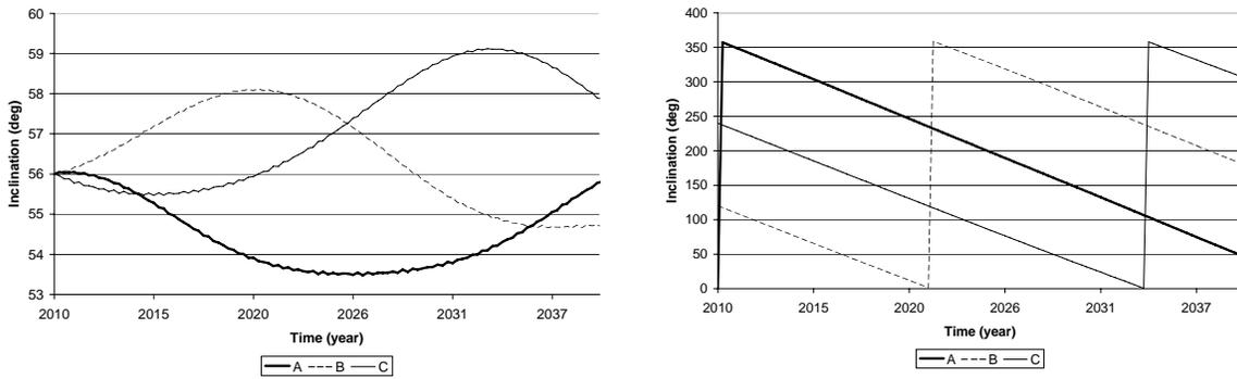
Fig 1. 20-year propagation. Inclination and RAAN values for satellites in each plane
