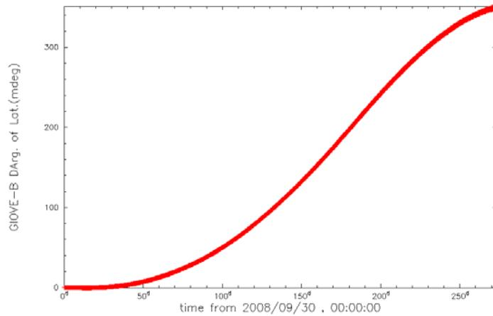
Fig. 11. Difference in argument of latitude between propagated orbit and sliding window orbit determination.
