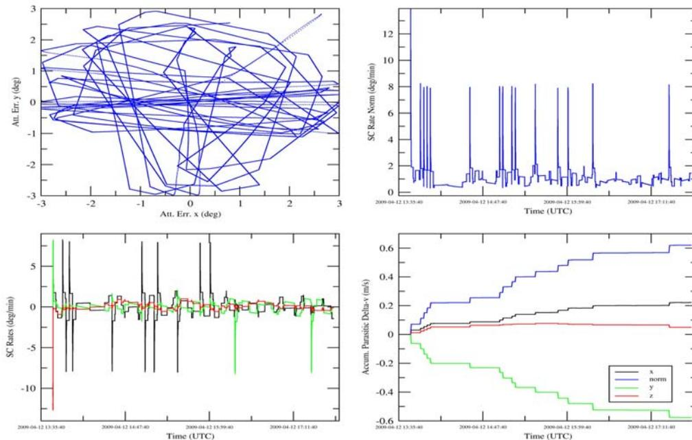
**Fig. 2 SAM controller behaviour from a HPTDG simulation after first OBDB parameter tuning**
