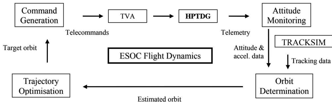
Fig. 1. ESOC FD subsystems and their main data interfaces during system tests
