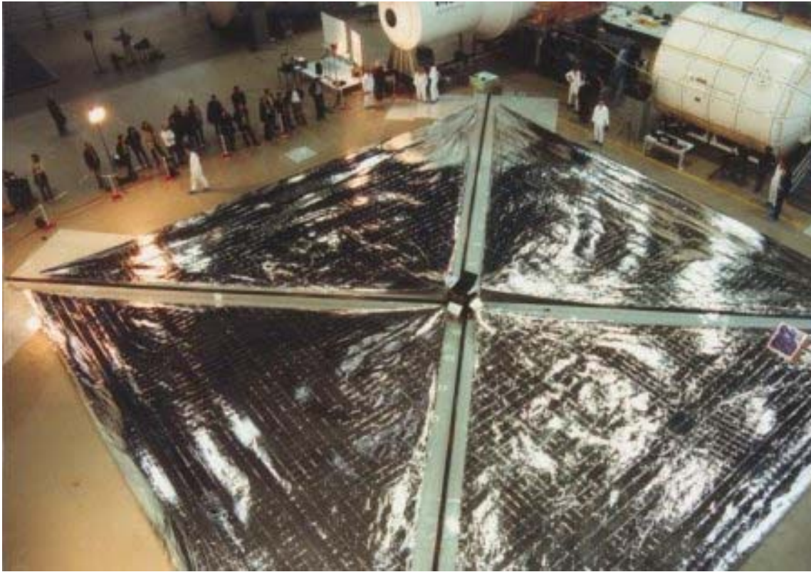
Figure 1. The 20-by-20 meters solar sail successfully deployed on ground by DLR in 1999
