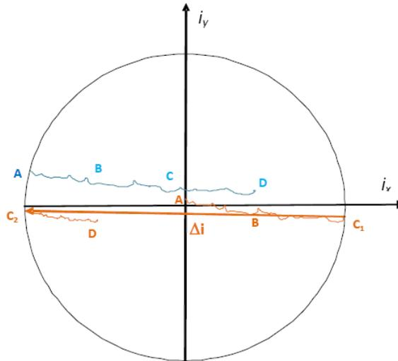
**Figure 2. Inclination Evolution of Collocated Satellite**
