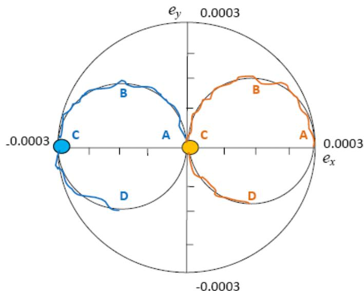
**Figure 7. Eccentricity Evolution of Collocated Satellites**
