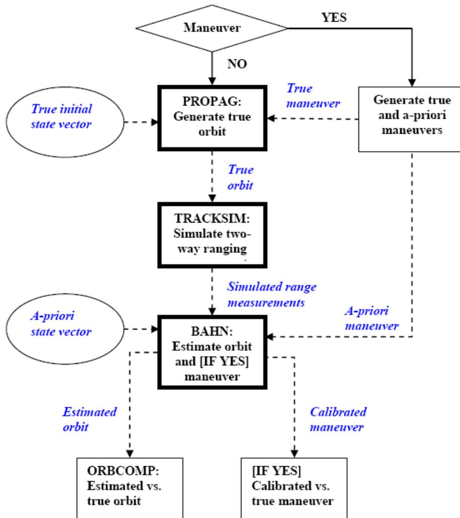
Figure 1. Orbit Determination Simulations Flow-Chart
