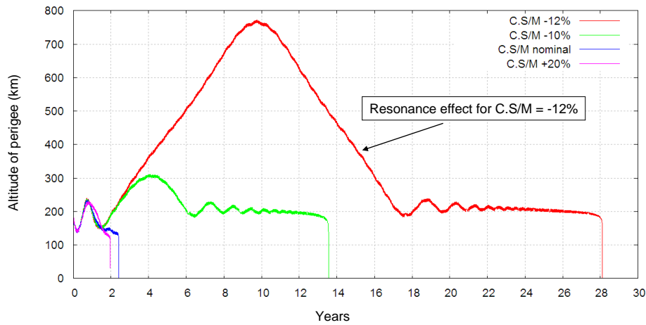
Figure 9. SPIRALE-A : Evolution of the perigee altitude for different values of drag ratio
