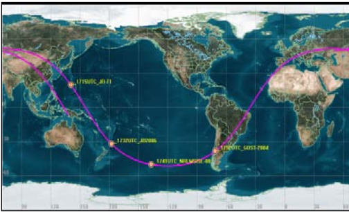
Figure 22. Fobos-Grunt reentry ground track issued approximately 1 hour before the probe decay
