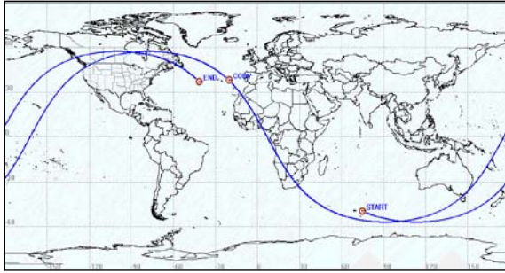
Figure 18. UARS reentry ground track issued 3 hours before the satellite decay
