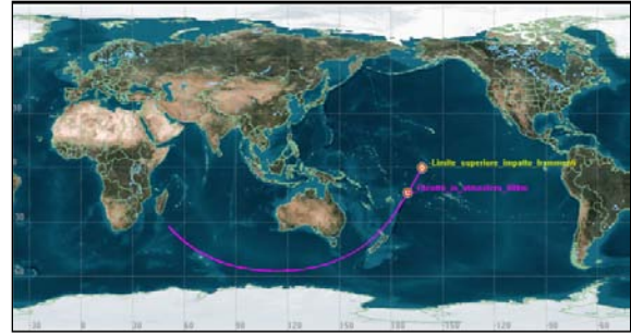
Figure 19. UARS final reentry ground track based on the JSpOC post-reentry assessment
