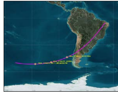
Figure 23. ISTI/CNR final assessment of the Fobos-Grunt reentry at the conventional altitude of 10 km
