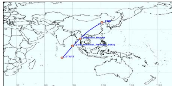
Figure 21. ROSAT final reentry ground track based on the JSpOC post-reentry estimation and uncertainties
