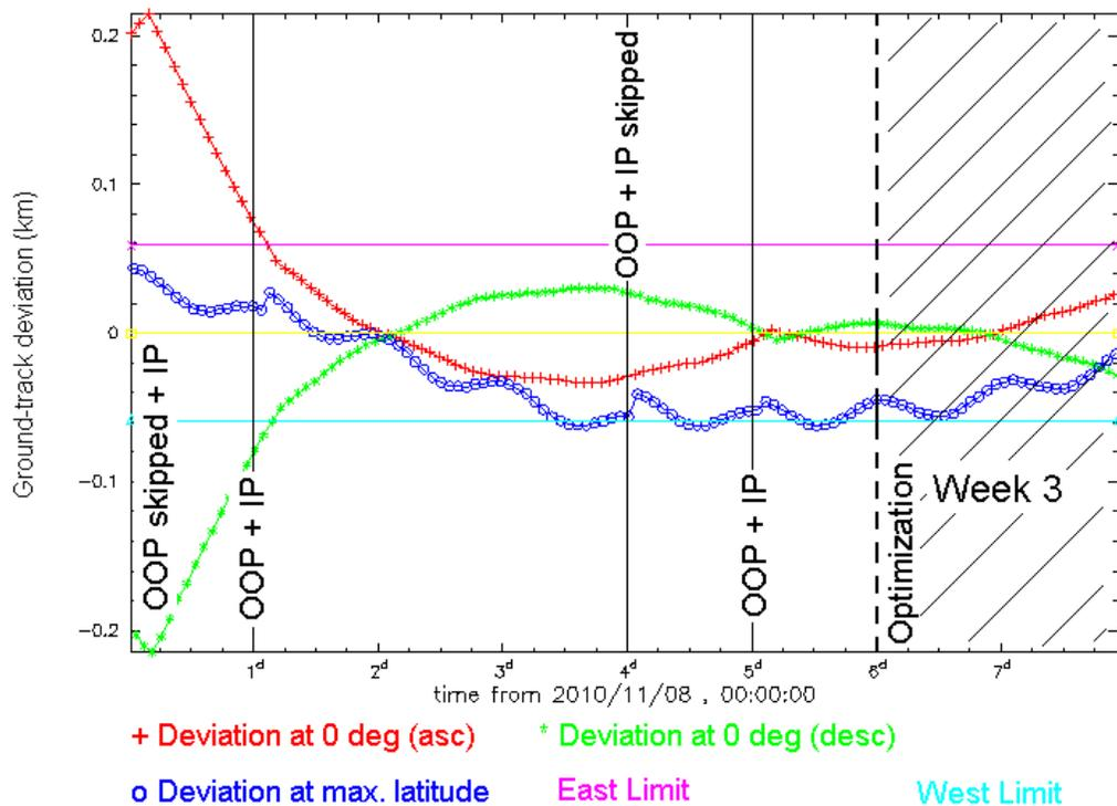
**Figure 4 Step 3: recovery after manoeuvre optimization on week (cycle) 2. Medium solar activity**
