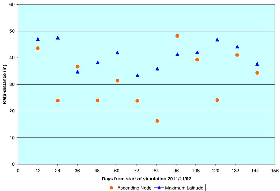
**Figure 9 RMS distance with respect to the Earth Fixed reference orbit**
