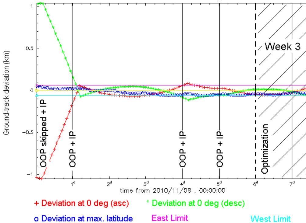
**Figure 7 Step 3: recovery after manoeuvre optimization on week (cycle) 2. High solar activity (+storm)**
