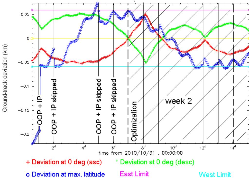
**Figure 2 Step 1: evolution of the ground-track deviation after manoeuvre optimization on week (cycle) 1. Medium solar activity**
