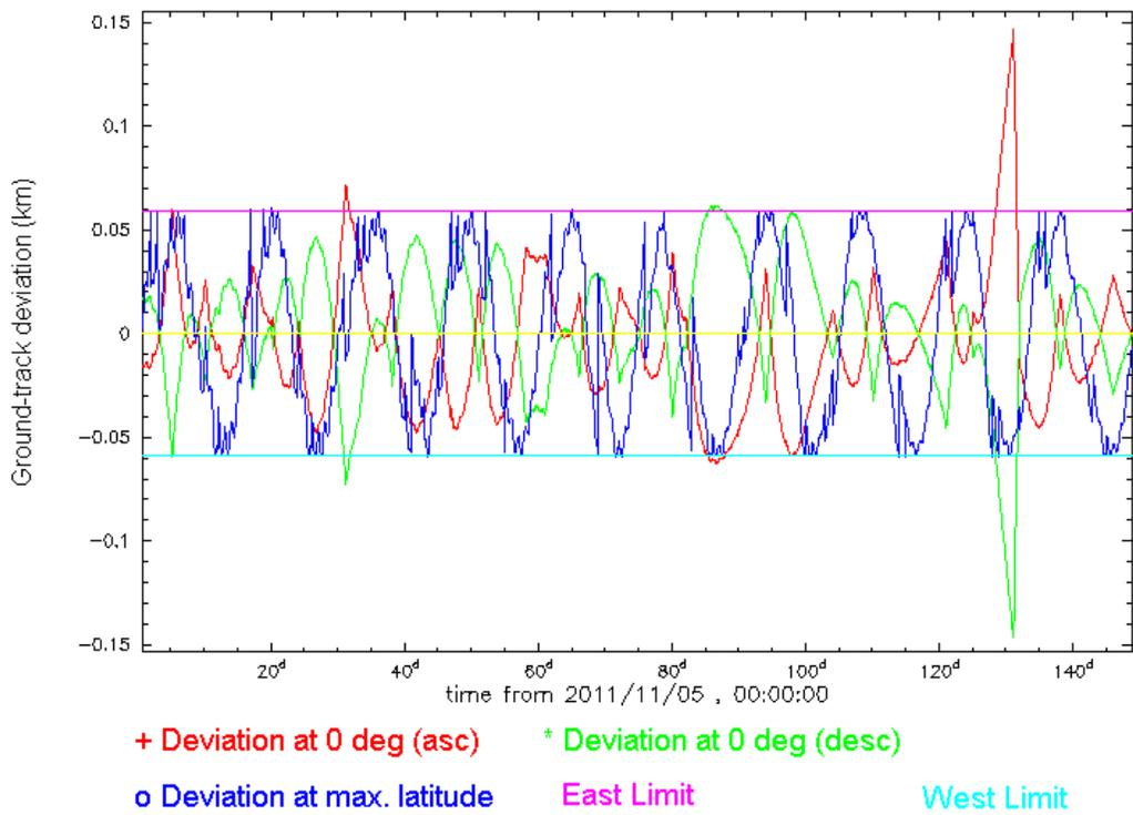
**Figure 8 Results of the nominal orbit control simulation. Ground-track deviation**
