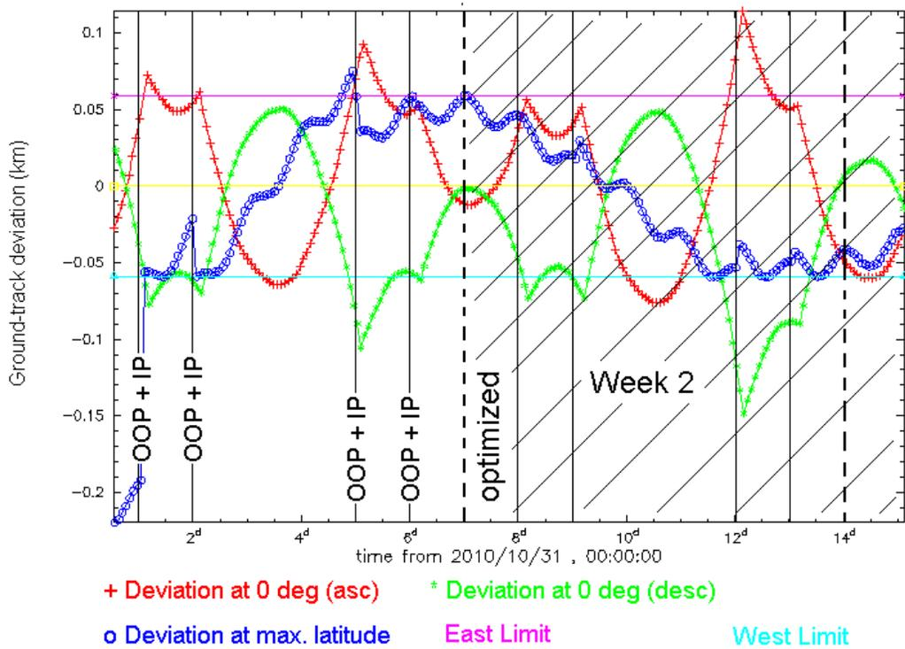
**Figure 5 Step 1: evolution of the ground-track deviation after manoeuvre optimization on week (cycle) 1. High solar activity (+ storm)**
