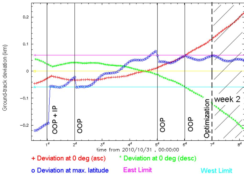
**Figure 3 Step 2: real ground-track evolution during week (cycle) 1. Medium solar activity**
