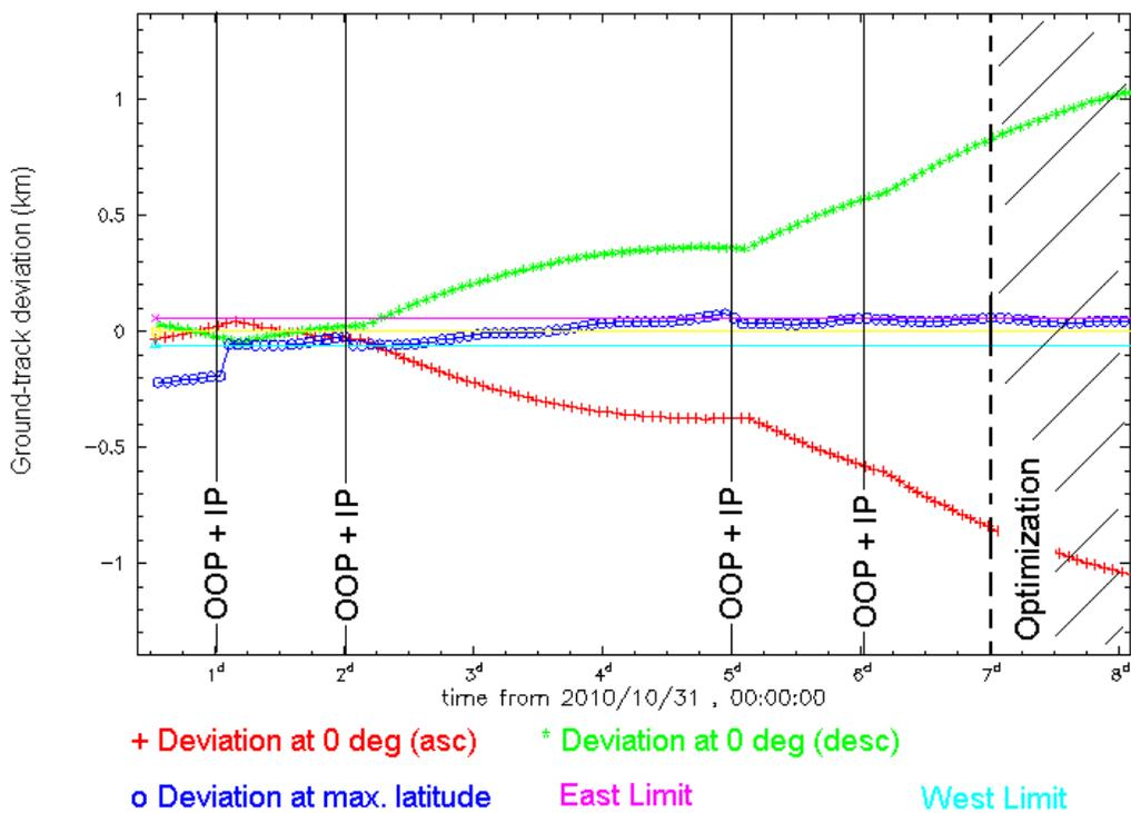
**Figure 6 Step 2: real ground-track evolution in week (cycle) 1. High solar activity (+ storm)**
