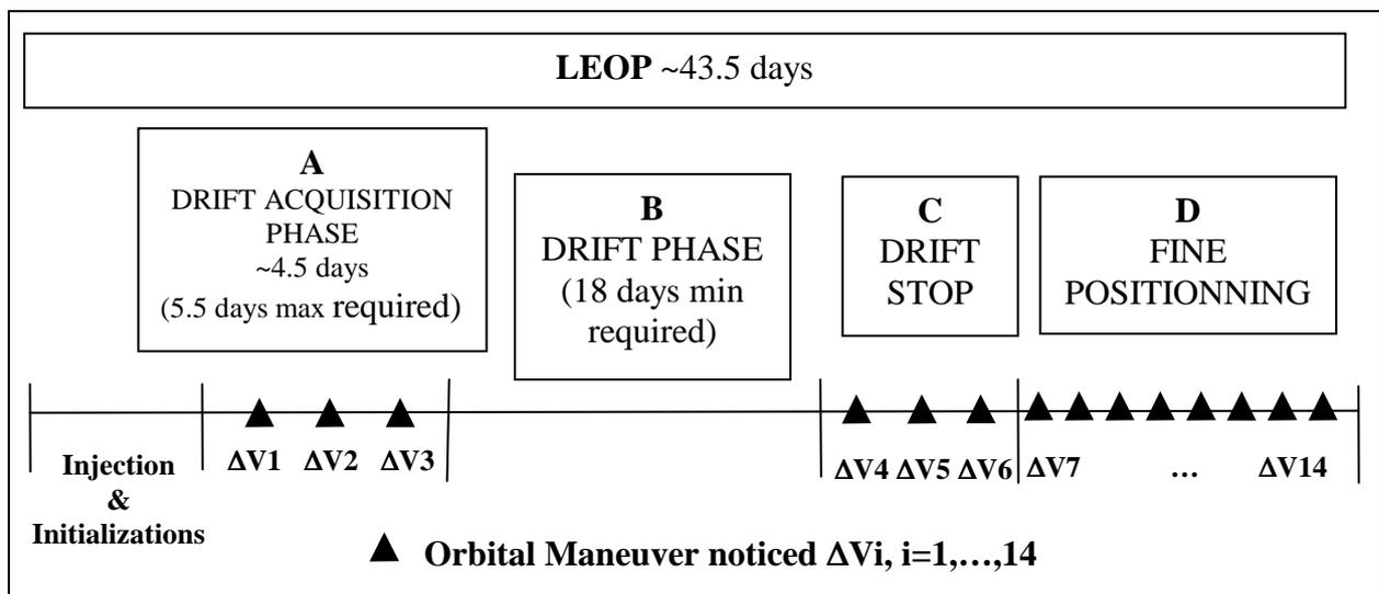
**Figure 1. Maneuver scenario with phasing constraints**
