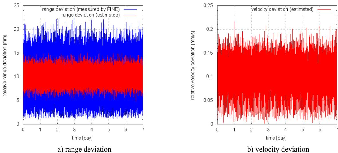
**Figure 5-2-1. Range & Velocity Deviations between Actual and Estimated Orbits**
