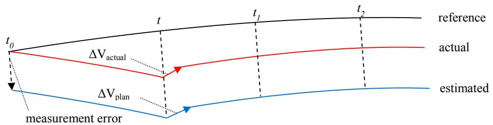
**Figure 4-1-1. Diagram of Relative Circular Orbit Keeping Control Law**
