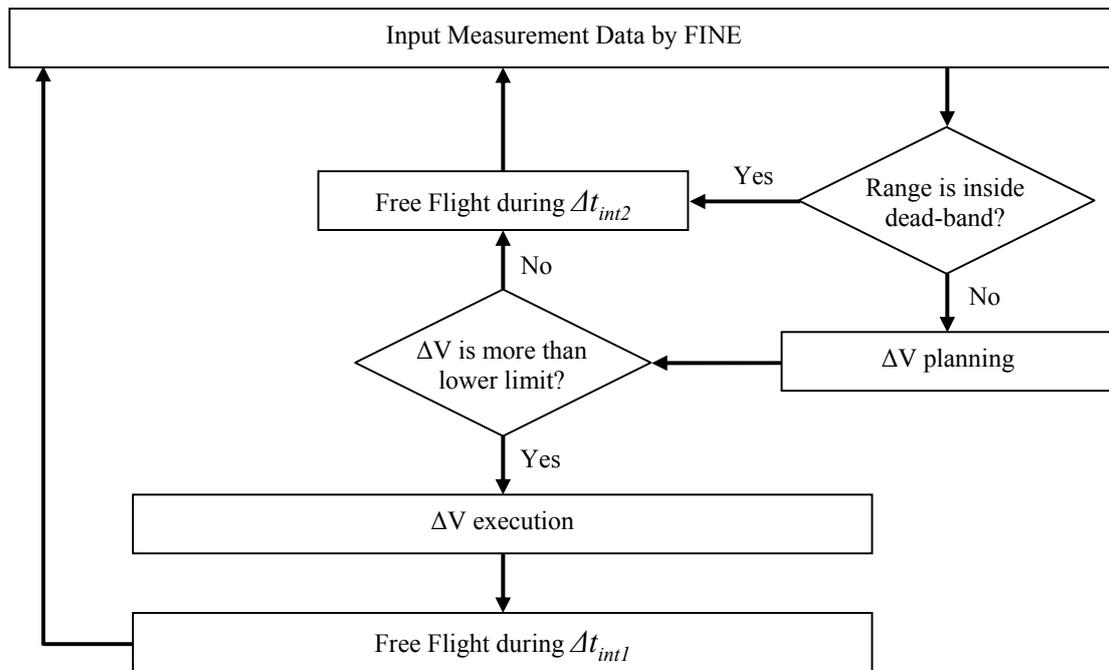
**Figure 4-1-2. Flow-Chart of Relative Circular Orbit Keeping Algorithm**
