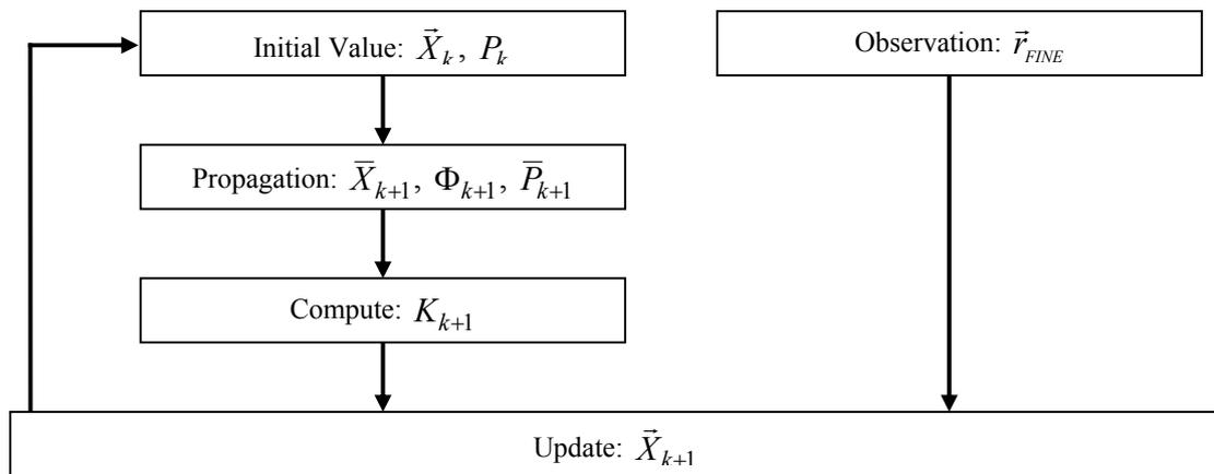
**Figure 4-2-1. Diagram of State Estimation Filtering**
