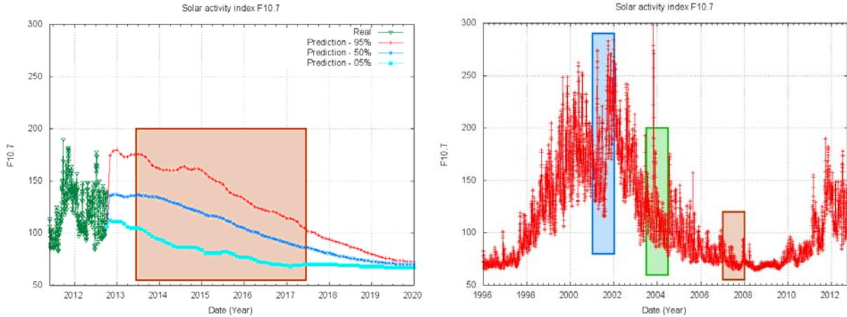
**Figure 4. *Left*: Predicted solar activity from 2012 to 2020. The shadowed area is the expected 4 years life from the beginning of the routine phase (June 2013). *Right*: Solar activity from 1996 to 2012. Shadowed areas are the chosen time span for the simulations, which are representative of the 95%, 50% and 5% of the solar activity predictions for the life of the mission. Blue is for high solar activity (95%), green for medium (50%), and brown for low (5%).**
