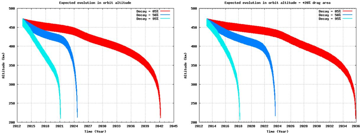
**Figure 2. Expected evolution of the altitude of the lower pair considering the solar activity predictions of the 5%, 50% and 95%. On the left with a nominal average drag area of 1.1 m<sup>2</sup>, on the right, with an area 20% higher.**
