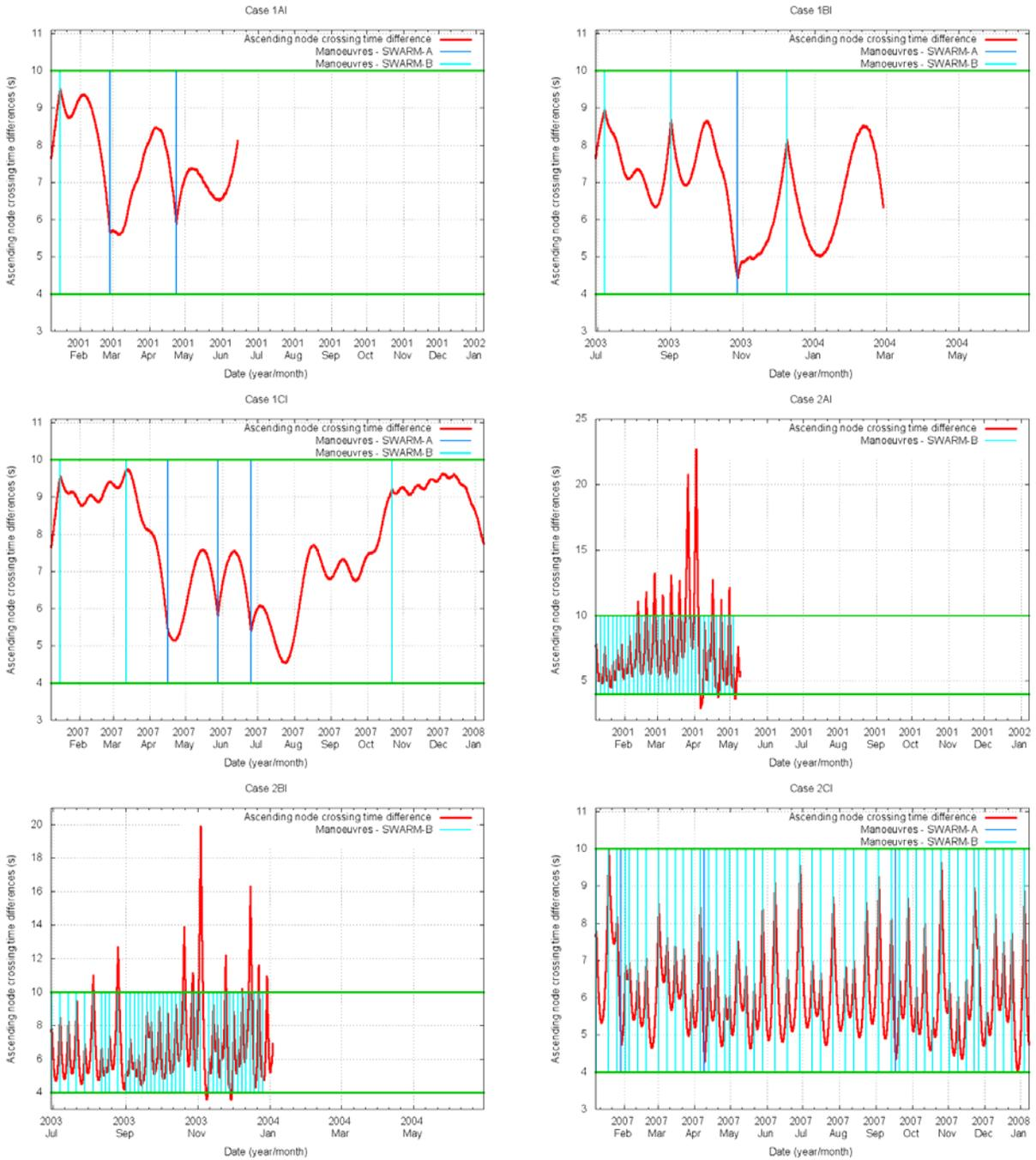
**Figure 6. Results of the simulations starting at 350 km in terms of  $dt$  evolution as a function of time. Vertical lines are manoeuvres. From top to bottom and left to right, cases 1A1, 1B1, 1C1, 2A1, 2B1 and 2C1.**
