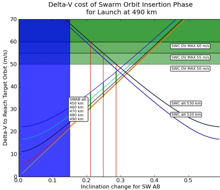
**Figure 1. Mission design diagram for the launch at 490 km. Blue and green shadowed areas are forbidden regions, and the different curves represent different altitudes for Swarm A/B/C.**
