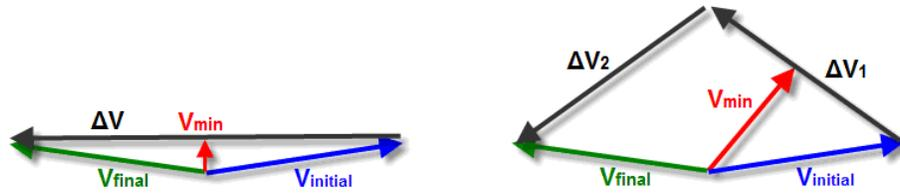
**Figure 6. Comparison of minimum velocity (in red) during 1-leg and 2-leg manoeuvres**
