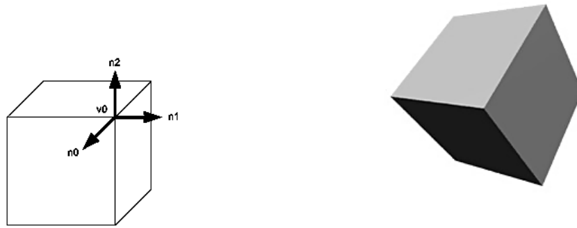
(a) Defining the cube face normals (b) OpenGL Rendering the shaded cube Figure 4: OpenGL Shaded cube
