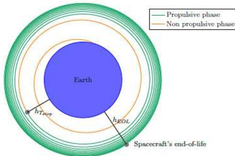
**Figure 2. Representation of a semi-controlled re-entry with low-thrusts**
