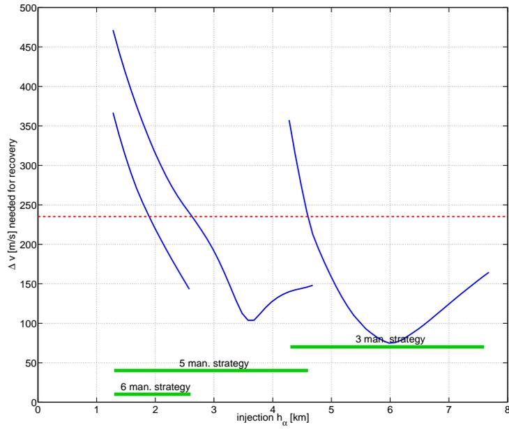
Figure 5. Transfer  $\Delta v$  for the various manoeuvre strategies explained in the text. The dashed line indicates the  $\Delta v$  available for recovery.
