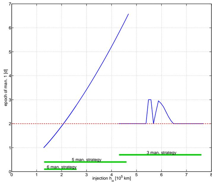
Figure 6. Time to first manoeuvre for the various manoeuvre strategies explained in the text. The dashed red line indicates the constraint of minimum 2 d applied to the 5 and 3 manoeuvre strategies.
