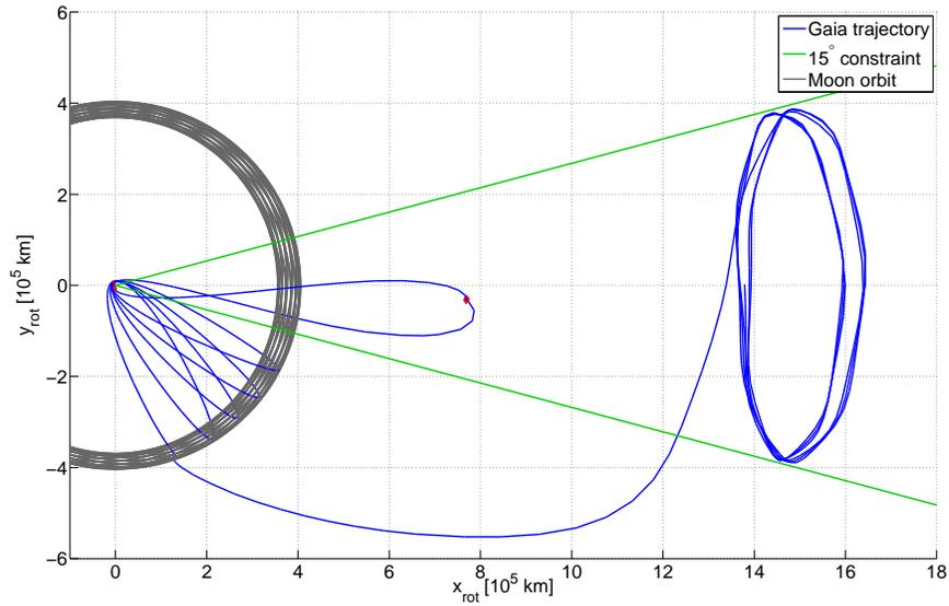
Figure 2. Trajectory of a successful 3 manoeuvre transfer to the target libration orbit after a severe underperformance launch failure resulting in a high apogee of 768,000 km. The transfer and target trajectories are shown in blue. The gray line represents the orbit of the Moon during the same time frame. The red markers indicate the locations of the 3 manoeuvres.
