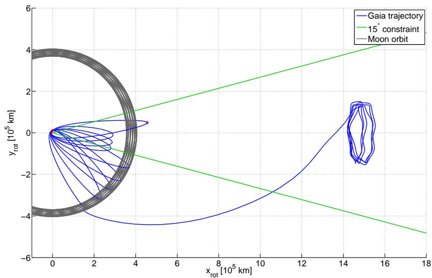
Figure 3. Trajectory of a successful 5 manoeuvre transfer to the target libration orbit after a severe underperformance launch failure resulting in a moderate apogee of 468,000 km. The transfer and target trajectories are shown in blue. The gray line represents the orbit of the Moon during the same time frame. The red markers indicate the locations of the 5 manoeuvres.
