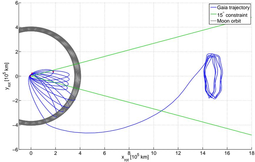
Figure 4. Trajectory of a successful 6 manoeuvre transfer to the target libration orbit after a severe underperformance launch failure resulting in a low apogee of 188,000 km. The transfer and target trajectories are shown in blue. The gray line represents the orbit of the Moon during the same time frame. The red markers indicate the locations of the 6 manoeuvres.
