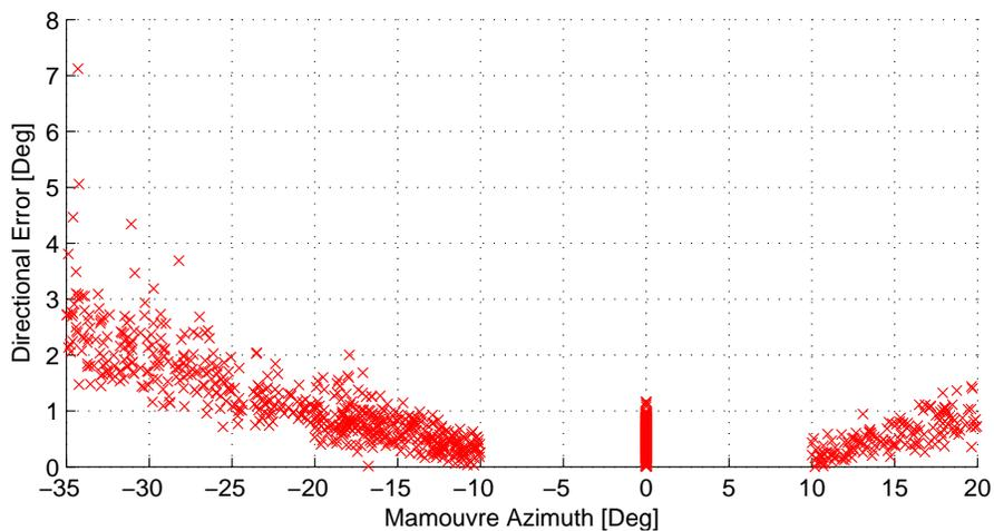
**Figure 7. Gaia directional manoeuvre error with respect to manoeuvre azimuth.**
