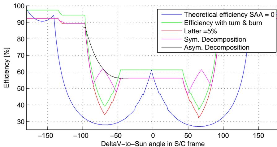
Figure 6. Manoeuvre efficiency dependant on  $\Delta V$ -to-Sun angle for different manoeuvre strategies for the Gaia chemical propulsion system configuration and Sun aspect angles between  $0-45^\circ$ .
