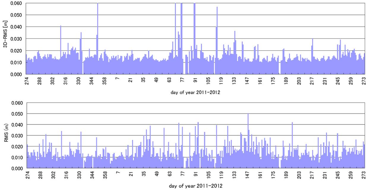
**Fig. 3 Daily position error in comparison with the JPL solutions (above) and SLR residuals (bottom) of GRACE-A with IAR on a year-round basis**
