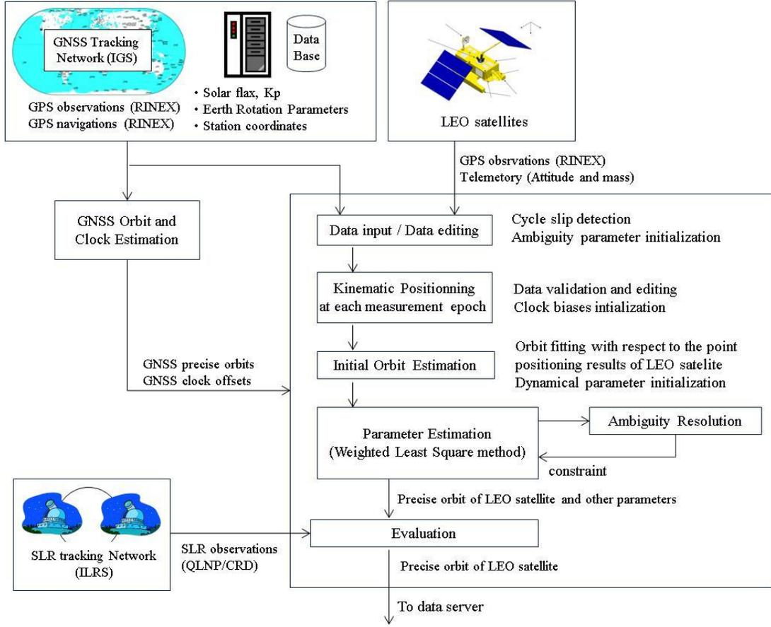
Fig. 1 POD software processing flow
