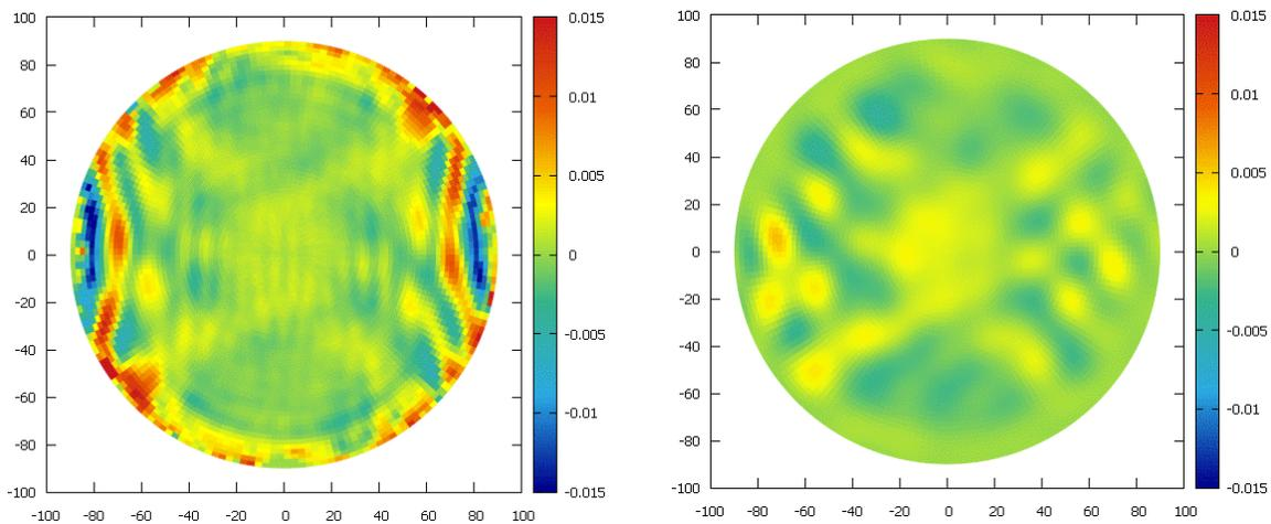
**Fig. 5 Empirical PCVs of GRACE-A antenna in meters with residual approach (left) and direct approach (right) on a year-round basis from 2011 to 2012**
