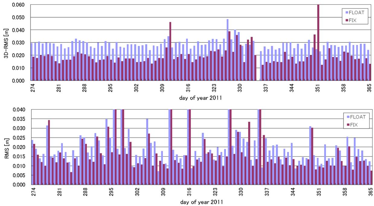
**Fig. 4 Daily position error in comparison with the JPL solutions (above) and SLR residuals (bottom) of GRACE-A WITH and WITHOUT IAR for 3 months**
