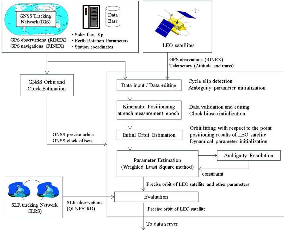
Fig. 1 POD software processing flow
