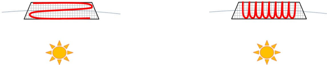
Fig 12. Scanning trade-off: first alongtrack, after radial (left), or first radial, after alongtrack (right)
