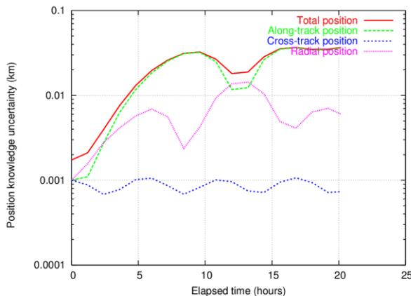
**Figure 1: Position knowledge uncertainty growth during operational delay interval**
