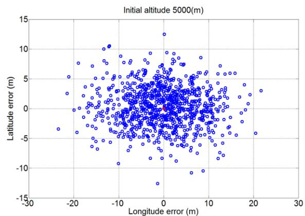
**Figure 2: Errors at Low-Gate from Monte Carlo simulation with fixed time terminal guidance**
