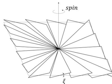
Fig. 2. Deformation model of spinning solar sail
