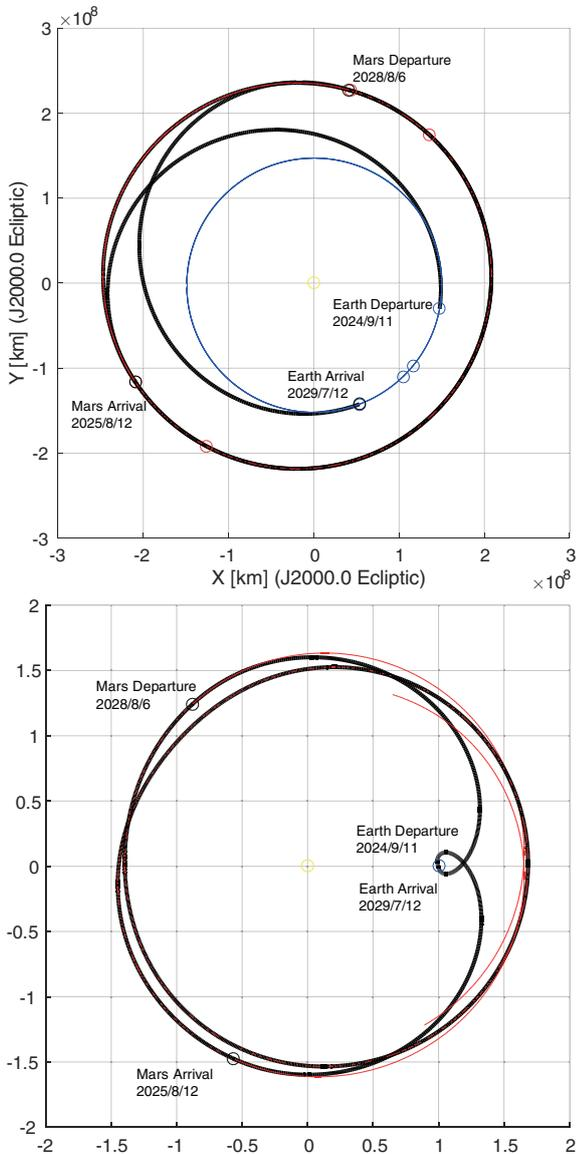
Fig. 1. An example for nominal interplanetary trajectories. Top: J2000 inertial frame. Bottom: Sun-Earth Fixed rotating frame.
