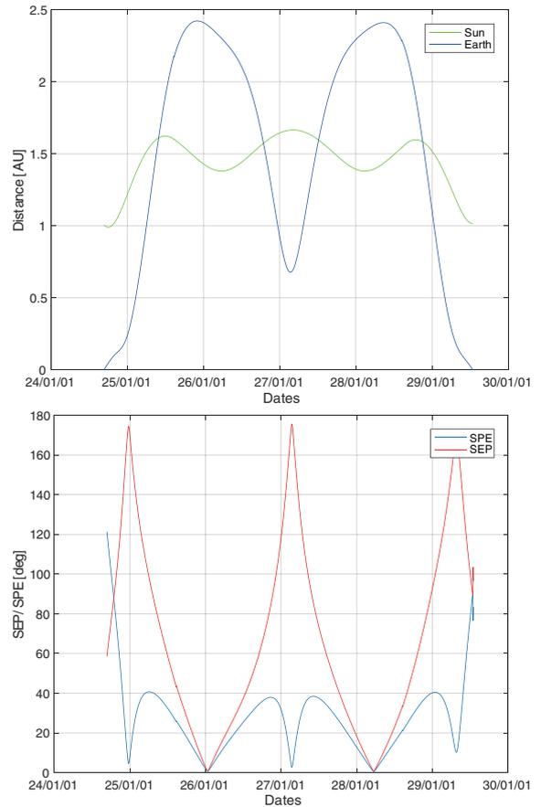
Fig. 2. Sun and Earth distance, Sun-Probe-Earth (SPE) angle, and Sun-Earth-Probe (SEP) angle (nominal).
