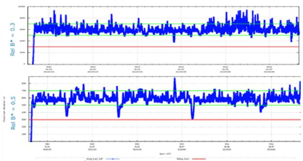
**Figure 8. Mirror manoeuvre long orbit control simulation results for two different relative ballistic coefficients: 0.3 (top) and 0.5 (down). Manoeuvre performance error 5% in magnitude and 1.5 deg in pointing at 1 sigma level.**
