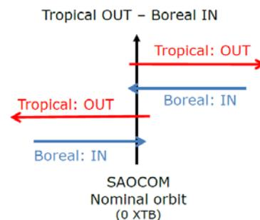
**Figure 3 Drift direction optimised for observation area**
