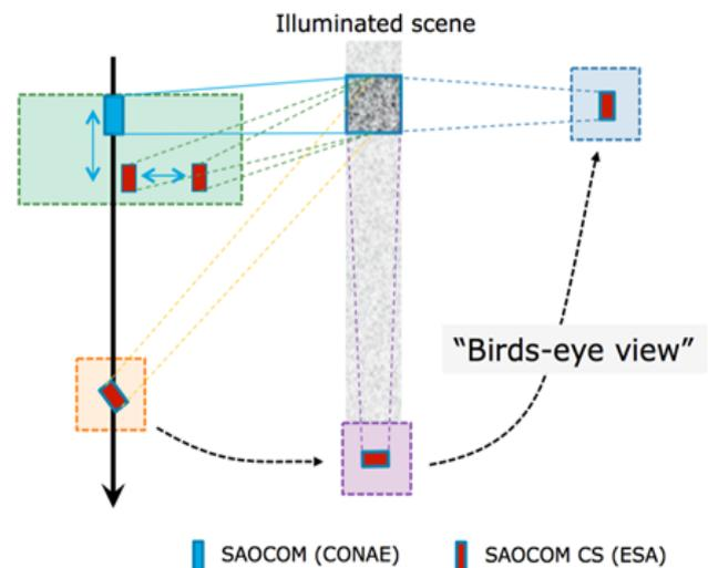
**Figure 1 SAOCOM-CS different geometries**
