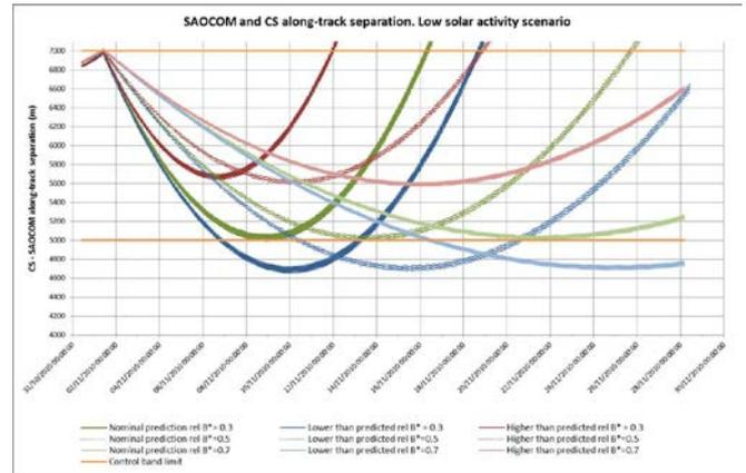
**Figure 5. Along-track separation evolution at low level of solar activity after propagation of a single manoeuvre.**
