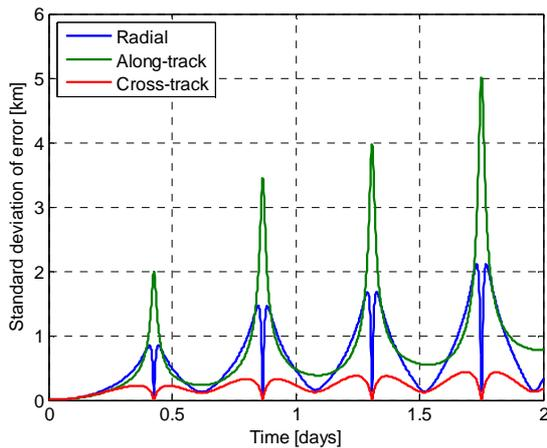
Fig. 4. Dispersions accumulated in radial, along-track and normal direction due to thrusting errors in the order of  $0.5^\circ$ ,  $1\sigma$  off-pointing
