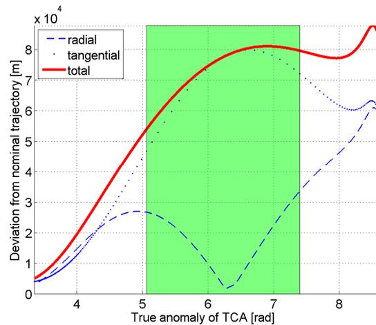
Fig. 7. Impact of switching the engine off for 30 minutes for various true anomalies. The deviation after exactly 12 hours is shown
