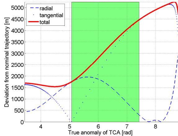
Fig. 6. Impact of switching the engine off for 30 minutes for various true anomalies. The deviation after exactly 2 hours is shown
