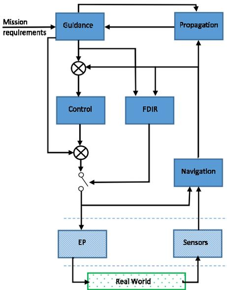
Fig. 1. Functional description of a Flight Dynamics system for transfer of Low Thrust satellites
