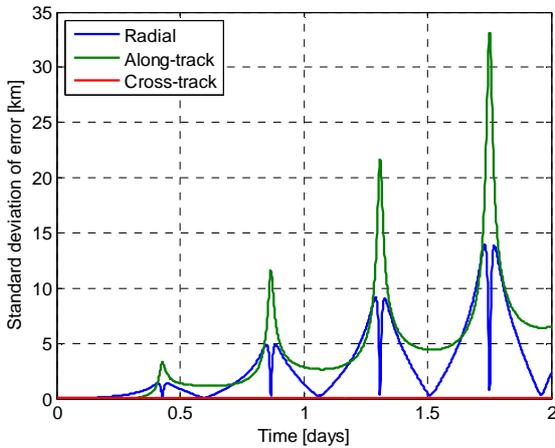
Fig. 3. Dispersions accumulated in radial, along-track and normal direction due to thrusting errors in the order of 0.5%,  $1\sigma$  thrust level
