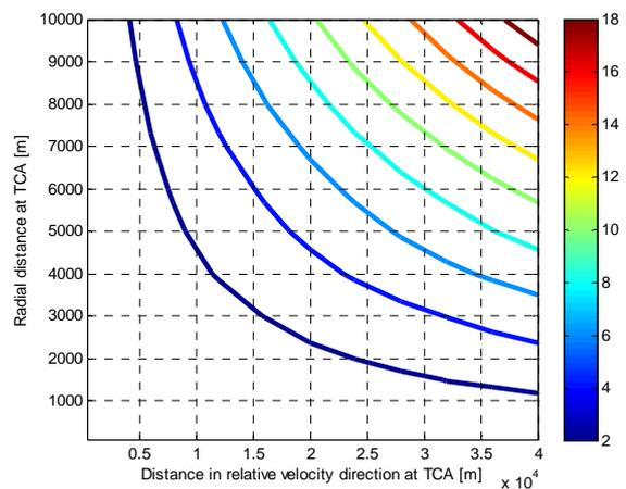
Fig. 5. Expected number of collision avoidance maneuvers as function of the radial distance and distance in the relative velocity direction at TCA.
