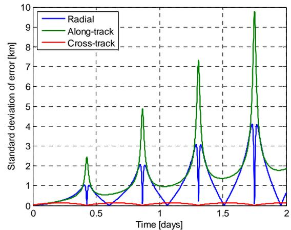
Fig. 2. Dispersions accumulated in radial, along-track and normal direction due to navigation errors in the order of 25 m & 2.5 cm/s,  $1\sigma$ , based on a full covariance matrix
