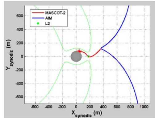
Fig. 5. AIM and MASCOT-2 trajectories in synodic frame
