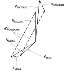
Fig. 9. Schematic of CAM triggering due to unexpected velocity
