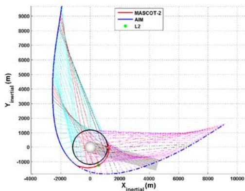
Fig. 4. Trajectories in inertial frame showing the line of sight from AIM to Didymoon (red: occultation by Didymain - black: eclipse – cyan: phase angle <90 deg – magenta: phase angle > 90 deg – solid lines: before release of MASCOT-2 – dashed lines: after release of MASCOT-2)
