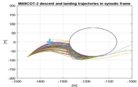
Fig. 6. Dispersion analysis of MASCOT-2 descent and landing trajectories in synodic frame
