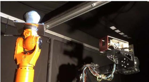
Fig. 10. Hardware-in-the-loop testing in robotic laboratory (image credits: GMV)
