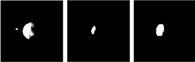
Fig. 8. Binarisation (left), erosion (centre), and dilation (right) for a sample navigation camera image of Didymos at 35 km (credits: GMV)
