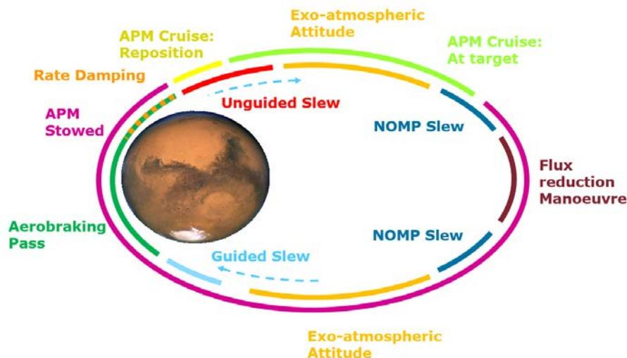
Fig 9. Timeline for an orbit a without manoeuvre with the HGA deployed and a FRM.
