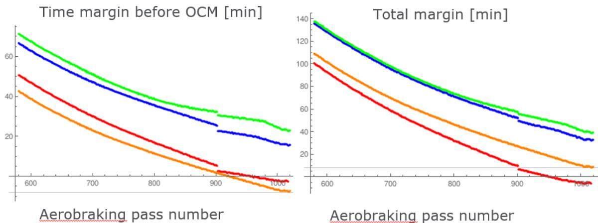
Fig 6. Time available before apocentre (left) and total time available in an orbit (right) in function of the aerobraking pass number and for different commanding strategies. Blue: pericentre raising manoeuvre using Long strategy (Fig 4) and Green using Short strategy (Fig 5). Red: pericentre lowering manoeuvre with Long strategy and orange with Short strategy.
