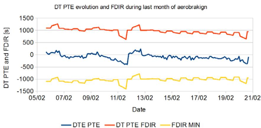
*Fig 7. In Blue DT PTE evolution during the last month of aerobraking. In Red and the Yellow the maximum and minimum deviation allowed.*
