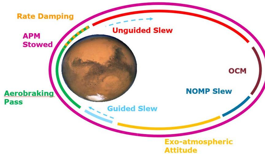
Fig 5. Orbit with a direct slew to the OCM and the slew back performed in thrusters.
