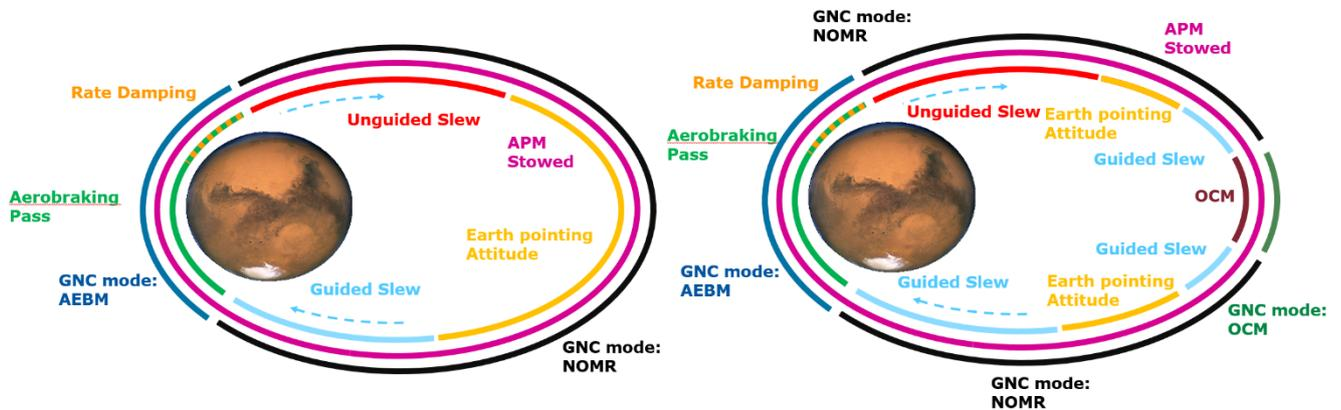
Fig 2: Right timeline for long orbits with manoeuvre (OCM) and left without.
