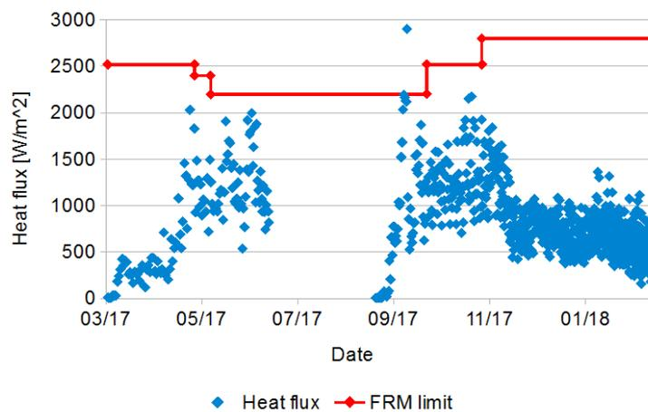
Fig 8. Reconstructed Heat flux and commanded threshold for FRM triggering.
