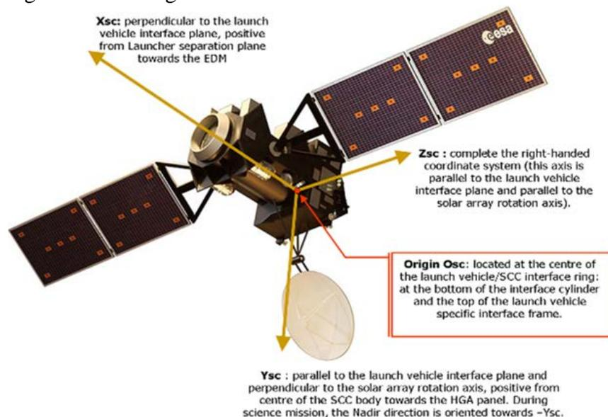
Fig 1: TGO reference frame definition without the EDM.
