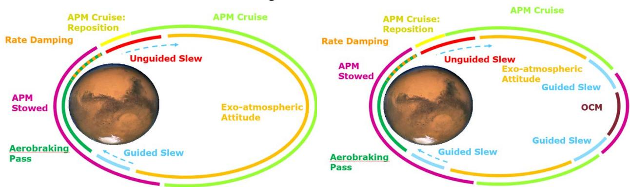
Fig 4: Timeline for short orbits with manoeuvre (right) and without (left). The GNC modes have been omitted for clarity purposes.
