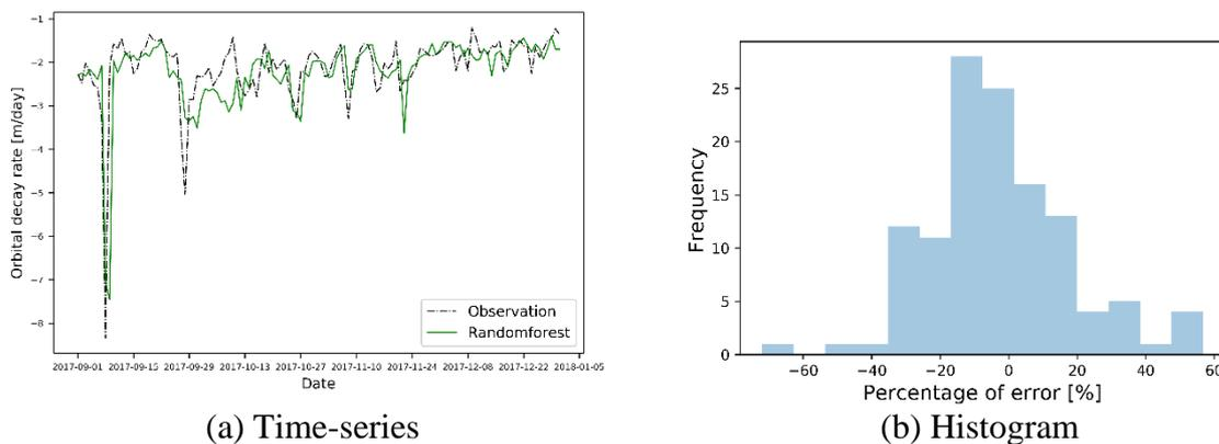
*Fig 2: Comparison of orbital decay rates between forecast model predictions and observations of the ALOS-2 satellite*
