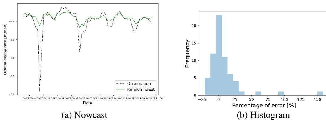
Fig 4: Comparison of orbital decay rates between forecast model predictions and observations of the GCOM-W1 satellite
