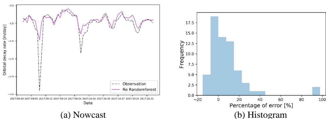
*Fig 3: Comparison of orbital decay rates between nowcast model predictions and observations of the GCOM-W1 satellite*
