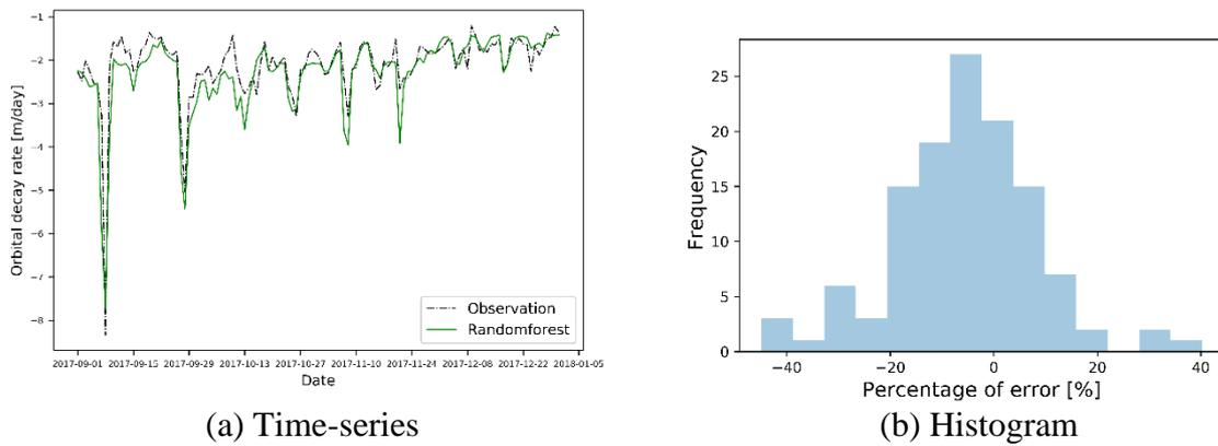
*Fig 1: Comparison of orbital decay rates between nowcast model predictions and observations of the ALOS-2 satellite*
