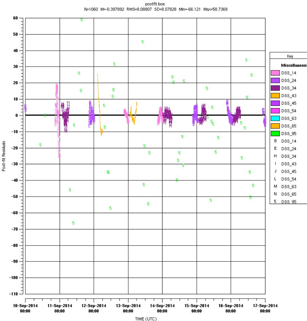
**Figure 11. DSN/IDSN Range Residual Comparison (Range Units) (IDSN=DSS-95, Green)**
