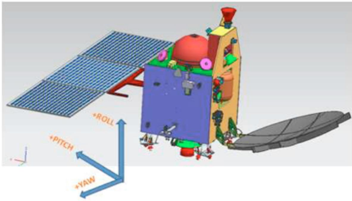
**Figure 7. MOM "On Orbit Configuration"**
