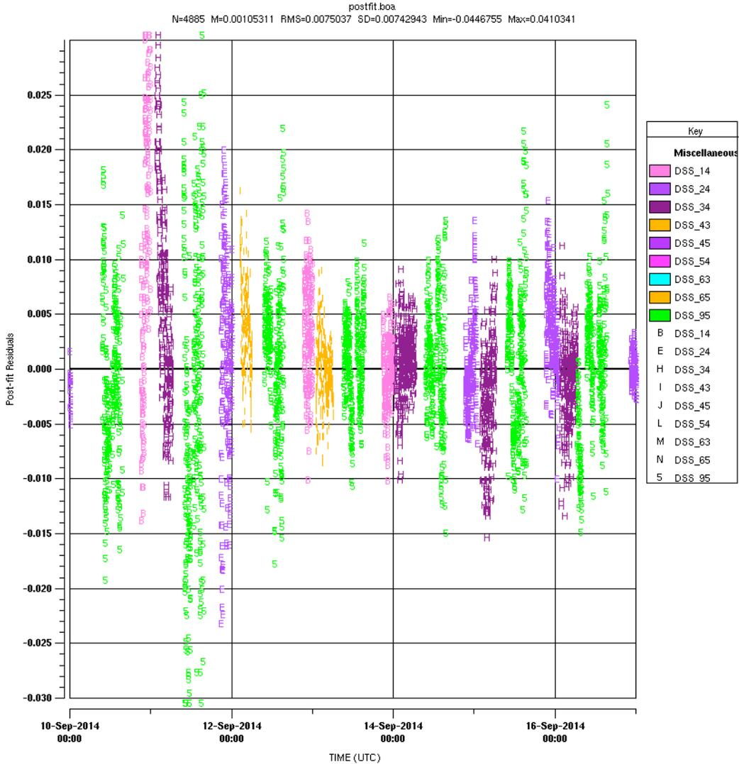
**Figure 10. DSN/IDSN Doppler Residual Comparison (Hz) (IDSN=DSS-95, Green)**
