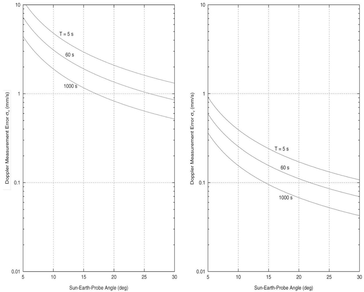
**Figure 3. Doppler Measurement Error (mm/s): S-up/down (left), X-up/down (right) [10]**
