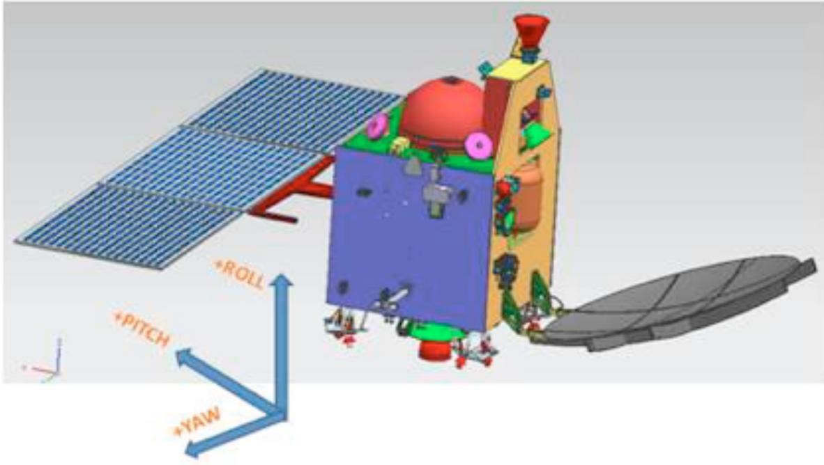
**Figure 7. MOM "On Orbit Configuration"**
