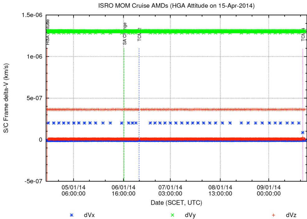
**Figure 8. MOM AMD Component-wise  $\Delta V$**
