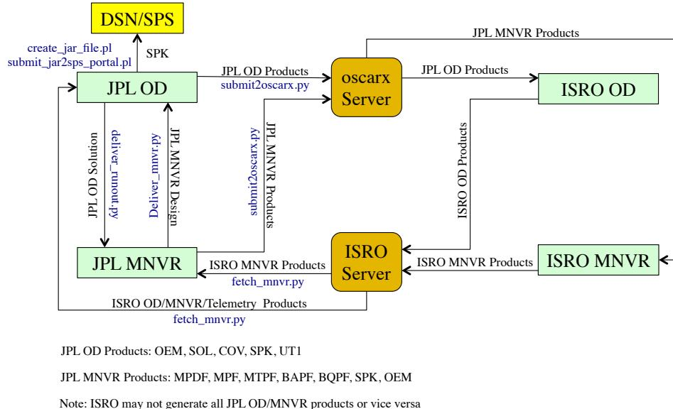
**Figure 1. Navigation Data Exchange Configuration**
