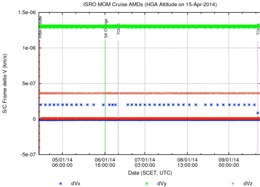
**Figure 8. MOM AMD Component-wise  $\Delta V$**
