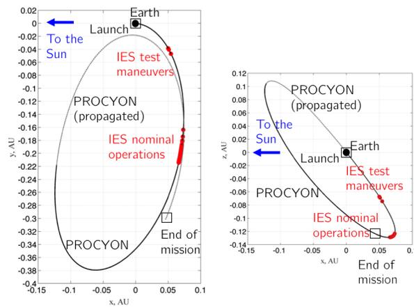
**Figure 2. PROCYON trajectory in the Sun-Earth rotating frame.**
