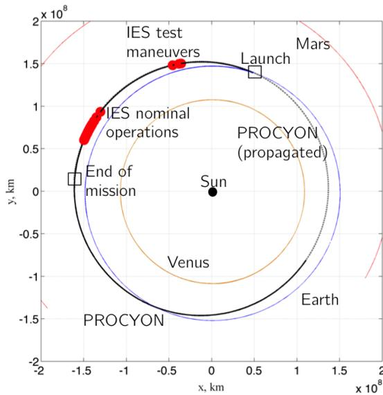
**Figure 1. PROCYON trajectory in the ecliptic J2000 reference frame.**
