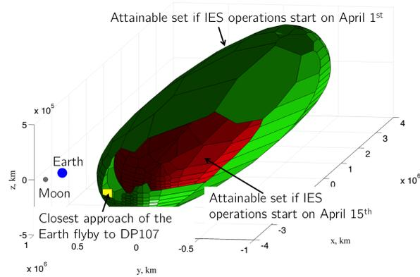
**Figure 13. Attainable set method used to compute the latest time of IES recovery to reach asteroid 2000 DP 107.**
