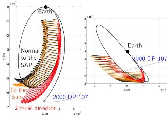
**Figure 9. Nominal trajectory to 2000 DP 107 in the Sun-Earth rotating frame.**
