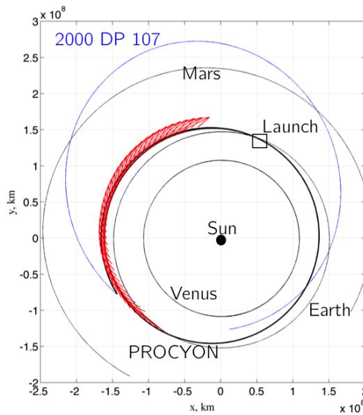
Figure 8. Nominal trajectory to 2000 DP 107 in the ecliptic J2000 reference frame.
