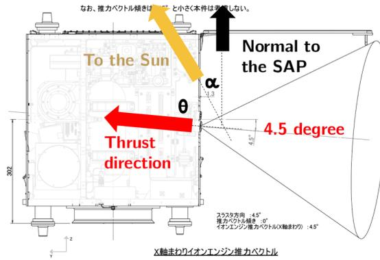
Figure 7. Power constraint and thrust direction.
