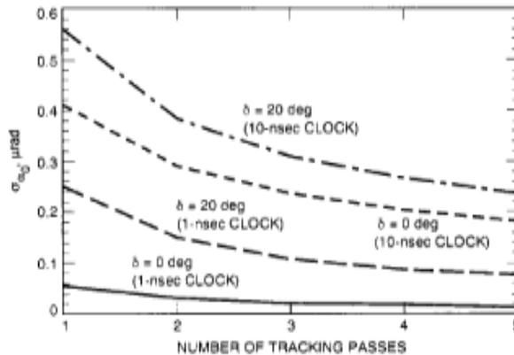
Figure 1. Comparison of USUDA -CANBERRA baseline declination for varying clock bias values
