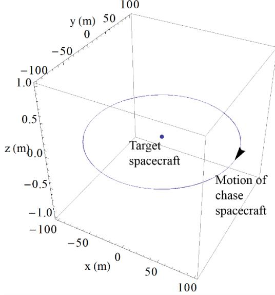
**Figure 5. Forced circular relative orbit using single-axis thrust.**
