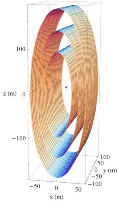
**Figure 3. Surface plot of possible chase spacecraft positions for  $-100\text{m} \leq y \leq 100\text{m}$ ,  $|a| = 1 \times 10^{-6} \text{ ms}^{-2}, 0.75 \times 10^{-6} \text{ ms}^{-2}, 0.5 \times 10^{-6} \text{ ms}^{-2}$ .**
